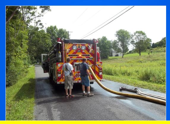
The goal of a tanker fill station is to operate much like a NASCAR pit stop. The large direct fill line and 5-inch LDH make a huge difference in fill time.
