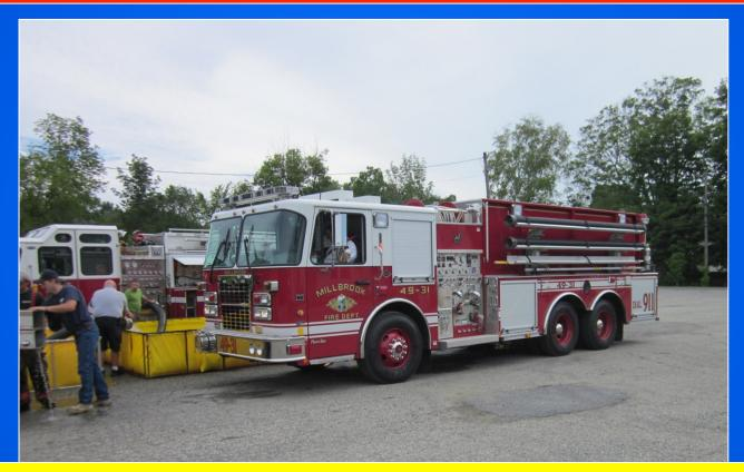
Tanker 49-31 uses a "cab-over" chassis design instead of a conventional/commercial chassis design which allows for a somewhat tighter turning radius..
