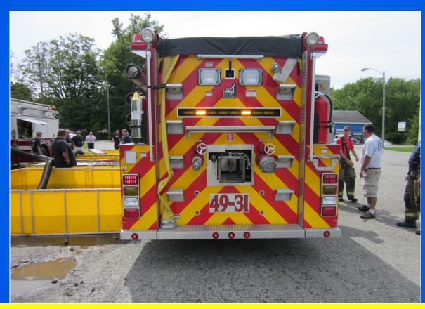
The business end of Millbrook's tanker has a 2-1/2" and a 5" direct fill in addition to a 10" square dump and plenty of scene lighting.
