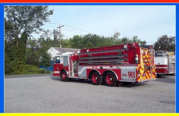
As noted many times, a rural rig can never have too much suction hose. Tanker 49-31 carries three, extra long lengths of 6-inch suction hose which can come in handy at many different drafting and dump tank operation scenarios.
