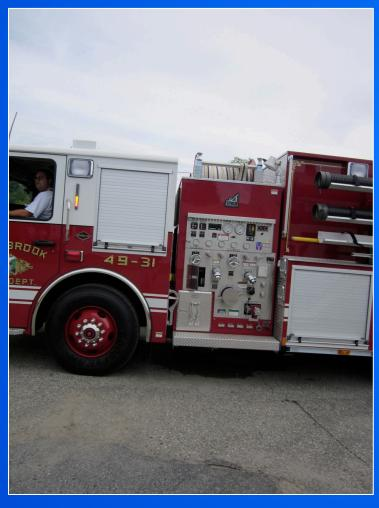
The 2,000 gpm pump provides plenty of pumping capacity if needed – thus making the tanker a versatile water supply unit either as a supply pumper, a nurse tanker, or a relay pumper. The tanker also has attack line stored on a reel in the dunnage area above the pump house.
