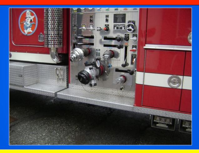
The pump on this rig is set-up to intake and discharge into 5-inch LDH.
