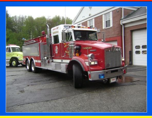
The use of the heavy-duty Kenworth chassis should provide a durable, long-life platform for this big water hauler.
