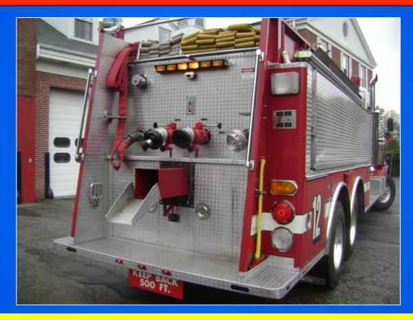
The business end of the engine/tanker is set-up to dump quickly and fill quickly – thus keeping this water hauler on the road.
