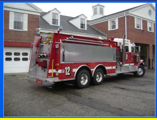
Tanker 12 is outfitted with a 10" dump in the teardrop area of the body on both sides and carries a 2,500-gallon dump tank.
