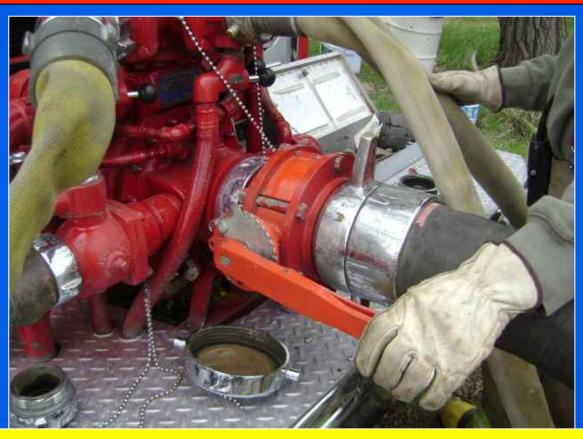
This pumper is also equipped with an external control valve on the suction intake. A suction intake valve is probably one of the best investments that a FD can make to enhance its drafting operations.
