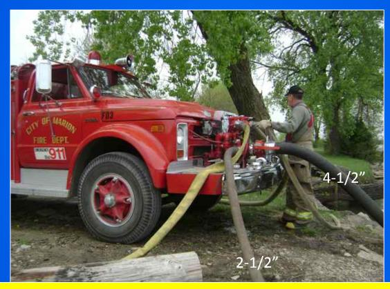
Engine 3 is shown here operating as a fill site pumper at a water supply drill in 2010. The experienced operator supplemented the 4-1/2" suction line by using a 2-1/2" "pony suction." Doing this increased the pumper's capacity to around 1,000 gpm.
