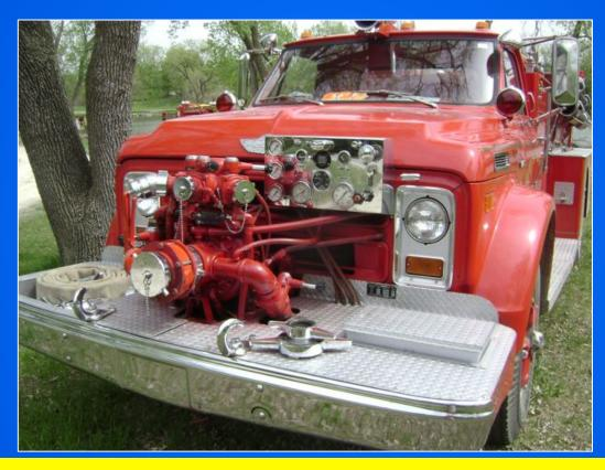
The front-mounted pump has been a mainstay of the rural fire service for many years. This type of pump configuration allows for easy access to drafting sites where space is limited.
