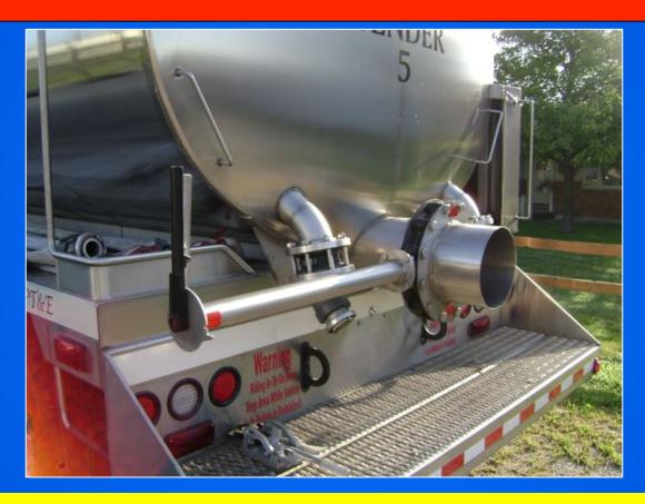
The 12" dump valve is a large, butterfly style valve that is manually controlled. Also – note the quick-connect fitting on the fill line – this reduces time spent making and breaking connections at the fill site.
