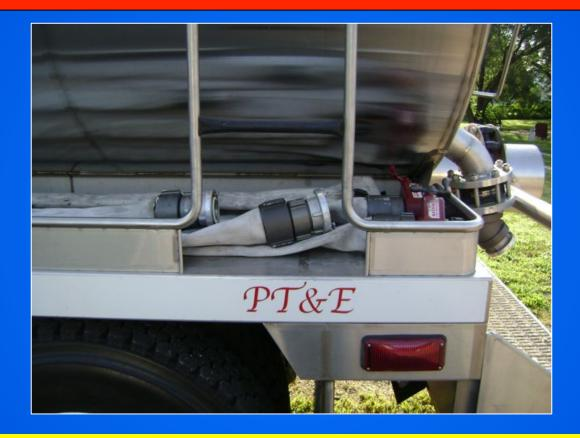
The tanker carries hose pre-rigged with valves and fittings for fill site operations. This is another time-saving measure that helps get the fill site up and running in a shorter time frame.
