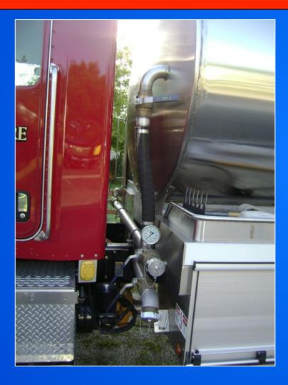
The tender is outfitted with an 800 gpm PTO driven fire pump which allows it to be used as a nurse tanker if needed until a dump site operation can be set up.
