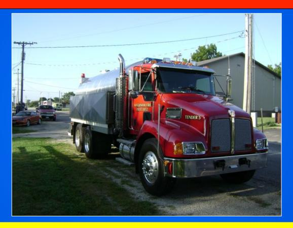
Tender 5 is a very simple rig that is set up to haul water from Point A to Point B in a very effective manner. Its 3500-gallon dump tank allows the water to be off-loaded and stored while the rig runs to get more.
