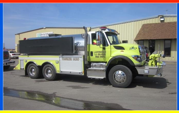
Tender 1430 carries a 3,000-gallon dump tank plus an assortment of water supply support equipment.
