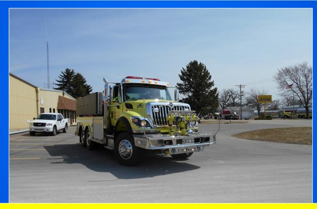
The rig is equipped with a 1,000 gpm Darley front mount pump making it more versatile in rural water supply operations. With a front mount pump the tender can work as a nurse tender, a supply pumper, or a relay pumper.
