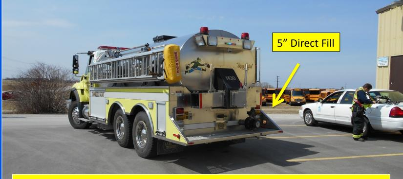
A 5-inch direct fill line is the standard fill line for all tenders in the mutual aid group to which Lauderdale-La Grange FD belongs. This standardized fitting plays a critical role in the success of large-scale water supply delivery operations like the 1,750 gpm drill in nearby Whitewater in April 2014.
