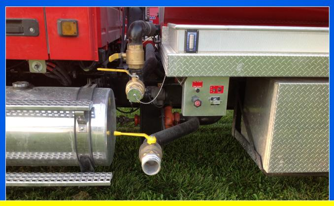
The tanker's 750 gpm pump is rather simple in design and layout. The pump allows the tanker to operate as a nurse tanker during the initial fire attack operation until such time that a dump site operation can be established.
