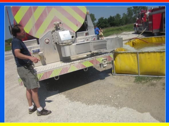
The swivel chute allows for side dumping with basically no loss in flow or offloading time. The Newton Swivel Chute can be retrofitted onto many older tankers.
