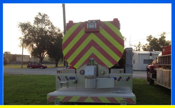
All of Tanker 3661's dumping occurs from the rear of the vehicle. It is equipped with a Newton Swivel Chute (kind of like a concrete mixer – ironic) which allows some flexibility in dumping. We wish to note that the tanker should be lettered on the rear so that the Water Supply Officer knows this is Tanker 3661.
