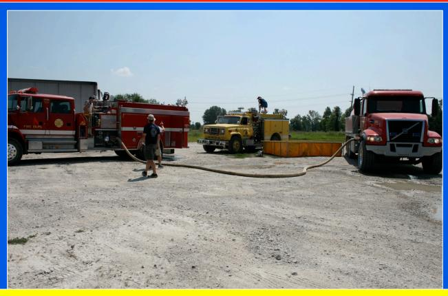
Tanker 3661 was the first arriving tanker at this 2-hr ISO drill and went into operation as a "nurse tanker" until the dump site could be set-up. Its 750 gpm pump made "all the difference. The drill supplied 500 gpm uninterrupted for 2-hours!
