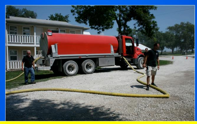
With only one direct fill line and only 3-inch hose available, the crew had to be creative in filling. The 3-inch lines were fed by a 5-inch line and they filled the tanker at 1,000-plus gpm.
