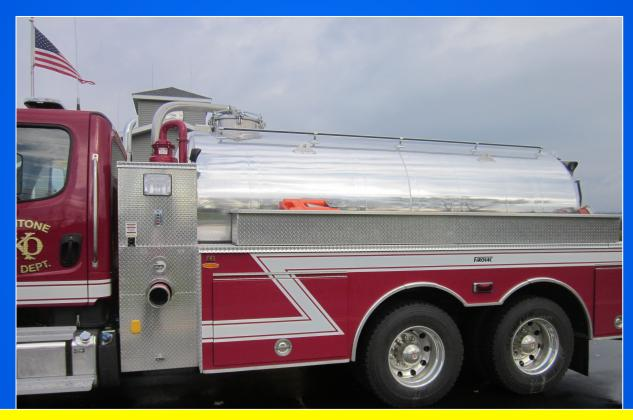
The tanker uses a 500 cfm vacuum for loading and off-loading its 2,600 gallons. The tanker has a 6-inch dump on both sides – which are also used as the loading ports.
