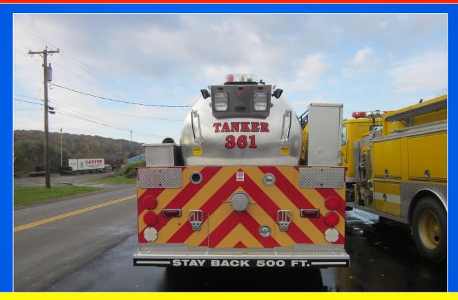
Nothing fancy on the rear — another 6-inch loading and off-loading port and a couple of compartments for suction hose and a strainer.
