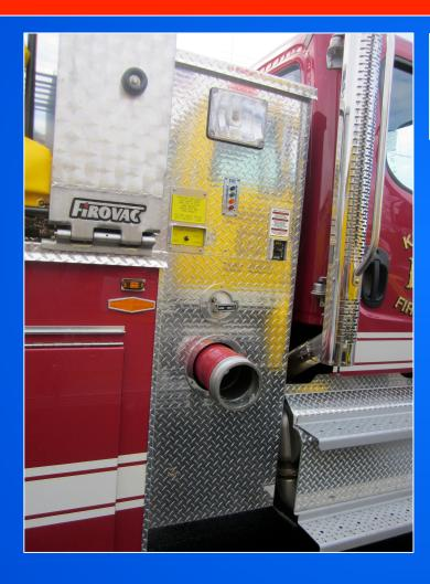
The tanker uses camlock style fittings to reduce the time spent making and breaking connections at the fill sites.
