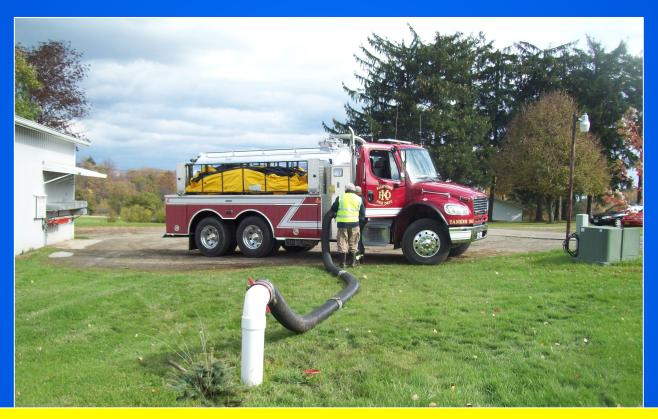
Tanker 361 is shown here "self-loading" from a dry fire hydrant at an October 2013 water supply drill in nearby Ashville, New York. Perhaps the greatest advantage of a vacuum tanker is its ability to load without the need for a pumper crew.
