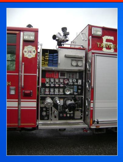
The panel on this engine-tanker is nicely laid out and looks to be operator friendly. The 2,000 gpm pump really makes the rig quite versatile as an attack engine, supply engine, or a nurse tanker.
