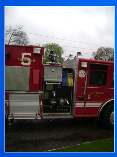
Tanker 6 has two, pre-connected crosslays and a pre-piped deck gun giving it some god fire fighting capabilities.
