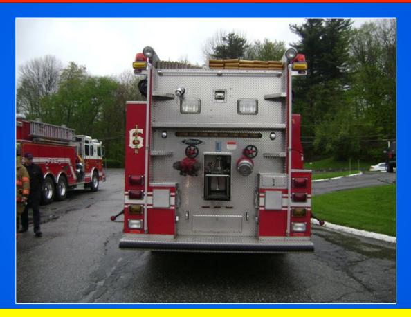
Tanker 6 is set-up with large-volume direct fill lines that will accommodate 5-inch hose.
