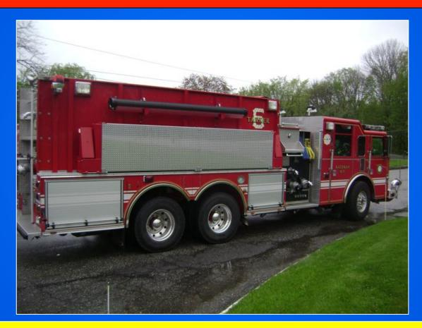
The 3,000 gallon dump tank allows for the tank to be emptied and the rig to get on the road for another load of water.
