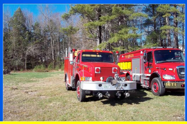
The front mount pump allows for easy access to static water sources. The manifold on the 1,000 gpm pump was fabricated and installed by the folks at the Jaffrey FD.
