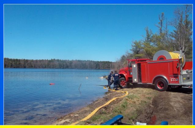
With a front mount pump, the reel truck can nose right up to the water's edge, thus minimizing lift. The rig's 4WD capability allows for easy exit as well.
