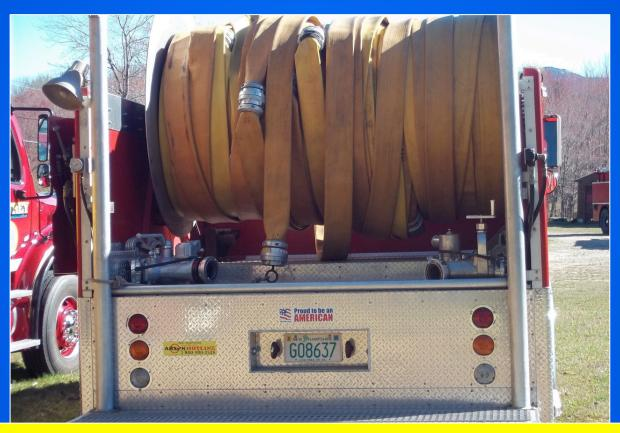
An LDH manifold and a Jaffrey Z-valve (in-line relay valve) are stored in readily accessible locations. The relay valve is important when trying to support large flows over long distances.
