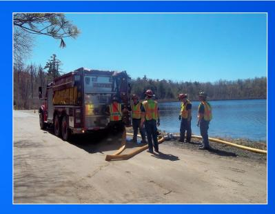
The crew from 16-Hose-1 operates a tanker fill site during this May 2013 water supply drill in nearby Rindge, New Hampshire. They were able to fill tankers at over 1,000 gpm using the reel pumper and 4-inch LDH.
