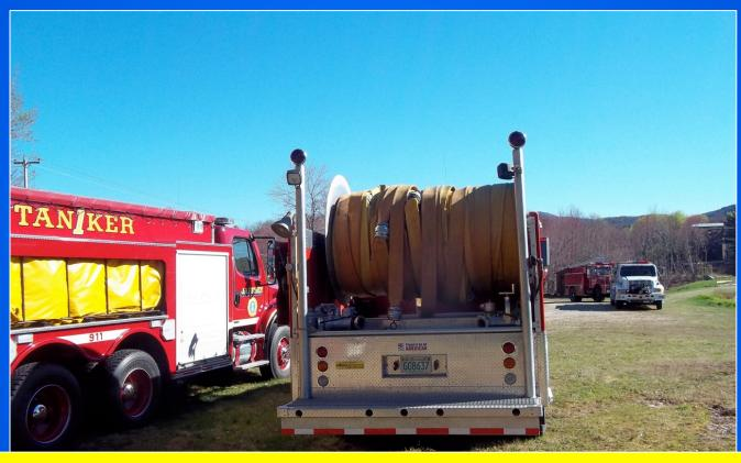
3,200-feet of 4-inch LDH is carried on a single hose reel. The reel is powered by a hydraulic system that is equipped with an electric clutch to control reel speed and motion.
