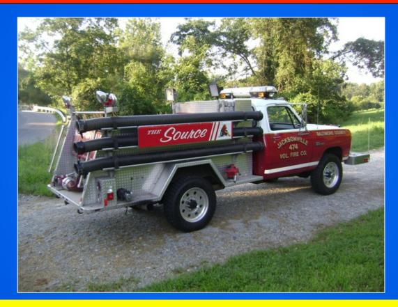
The TSU carries several lengths of suction hose plus the needed strainers and fittings to address a number of drafting scenarios.
