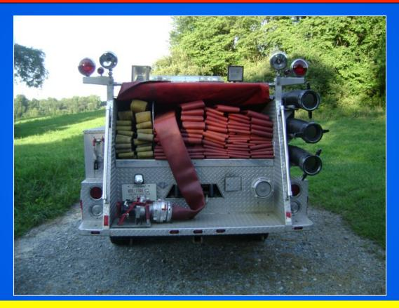
The 1,000 feet of 5-inch hose is trimmed out with a manifold which allows the driver to lay from the tanker fill site to the water source. Note the rear discharge on the lower right side of the vehicle.
