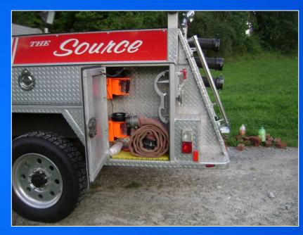
While the unit is nothing fancy, it is set-up to handle the ever important tanker fill operation. And for that scenario – this small package can deliver some big water.
