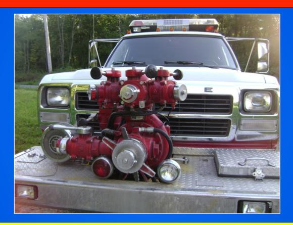
TSU 474's front mounted pump and 4-wheel drive capability make it an excellent rig for accessing remote water sources not reachable by a traditional pumper.
