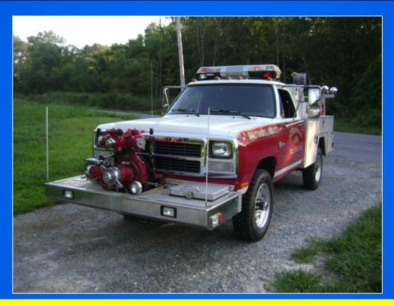
TSU 474 is know as "The Source" and its primary purpose is to draft water from ponds, streams and other sources in order to tanker fill site and support fire fighting operations.
