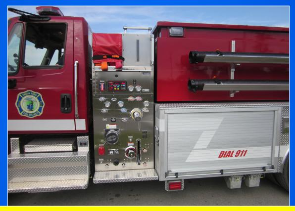
The 750 gpm Hale pump is PTO driven and allows the tanker to support a "nurse tanker" operation if needed during the early stages of fire attack.
