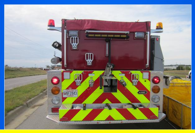
The tanker has 10-inch side and rear dumps and dual, 2-1/2-inch direct fill lines using Fireman's Friend Valves.
