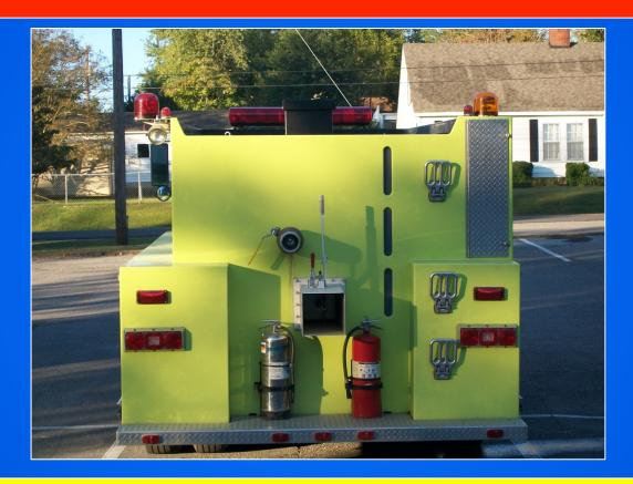
The tanker has a simple rear end as well – a 10-inch dump, a 4-inch direct fill, and a compartment for the 2,000-gallon dump tank.
