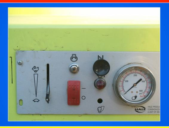
The pump is a small Hale pump that has a separate engine drive and very simple controls.
