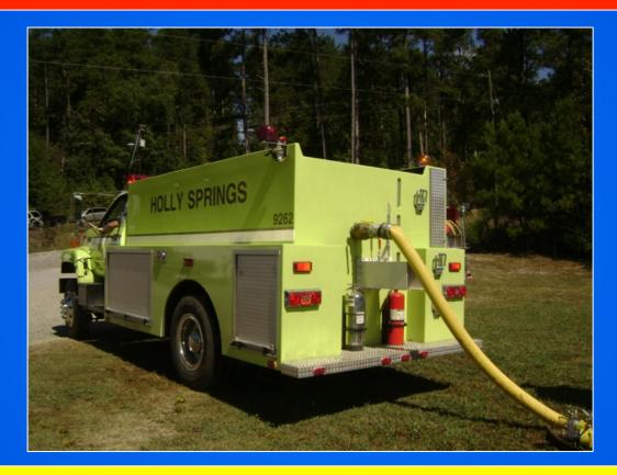
The 4-inch direct fill is equipped with a Cam Lock fitting for quick turnaround time at the tanker fill site.
