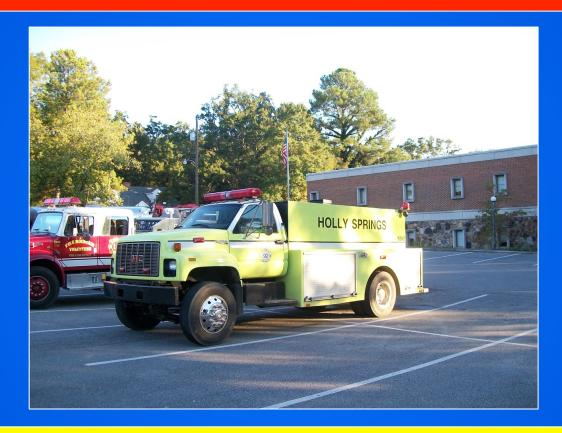
Tanker 9262 is set up to operate as a water hauling unit in a tanker shuttle operation. It has a 250 gpm pump for small scale operational support such as brush/woods fires.
