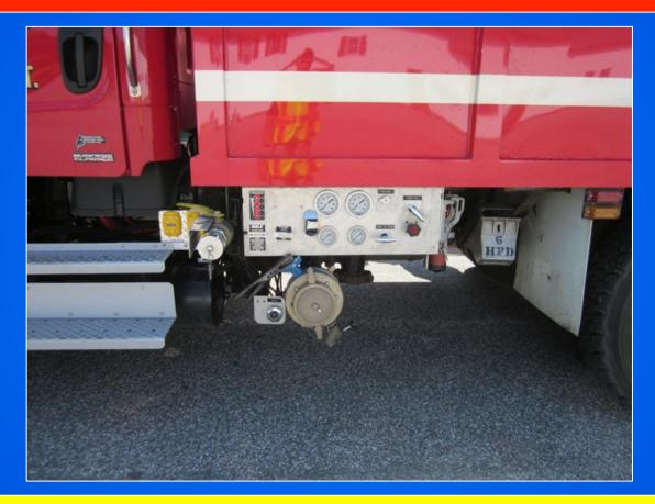
The tanker's 500 gpm PTO driven fire pump allows it to serve in a "nurse-tanker" mode – in a limited capacity –if needed.
