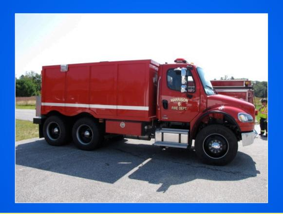
The 3,000-gallon tank is a poly tank. The tanker has limited compartment space – but that is okay because its job is to haul water.
