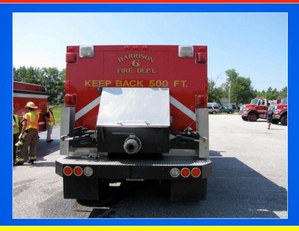
The tanker has a large, direct fill line on the rear (4-inch) that allows for a quick turnaround time at a fill site.
