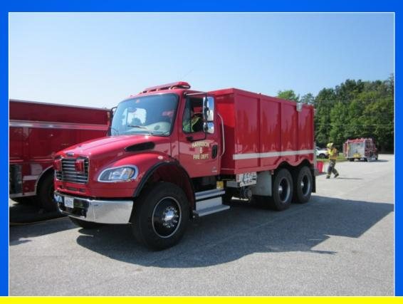
Tank 6 is a nice, short wheel-based 3,000-gallon tanker whose primary job is hauling water. The short wheel-base makes it perfect for the winding roads of the Lakes Region.
