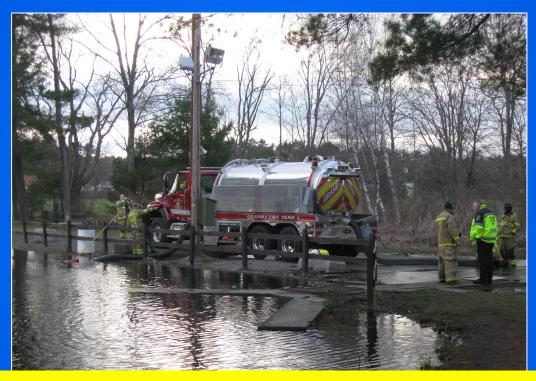
Perhaps the greatest advantage of a vacuum tanker is the ability to load using only one person. In a limited staffing situation such as Granby's – this feature plays a huge role in successful water supply operations. This vacuum tanker can load in excess of 1,000 gpm using any of its three inlets.
