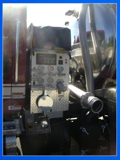
A nice feature of this tanker is its 1,250 gpm PTO driven pump. The pump provides added flexibility as well as ISO credit for pumping capacity. The PTO drive is becoming more and more popular as technology improves. In the past, the PTO option often was limited to a smaller 500 to 750 gpm pump. Today, PTO driven pumps can be found all the way up to 1,500 gpm.
