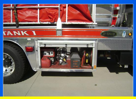
The tanker carries a limited amount of equipment - its primary focus is hauling water.
