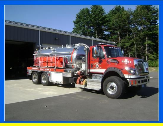
Tank 1 – like many vacuum tankers is equipped with two dump tanks. One for dump site operations and one that can be used for fill site operations.
