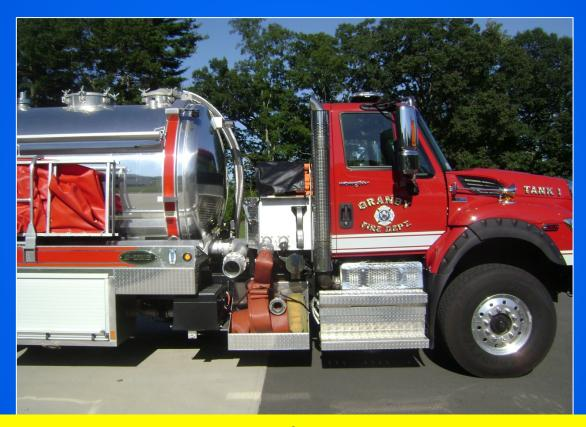
Tank 1 is equipped with a traditional fire pump so that it can serve as a nurse tanker if needed and pump off its water to an attack engine through supply hose.
