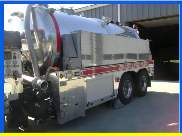
The tank on this rig is a 3,500-gallon aluminum tank that receives full credit under ISO because it is a sealed container.
