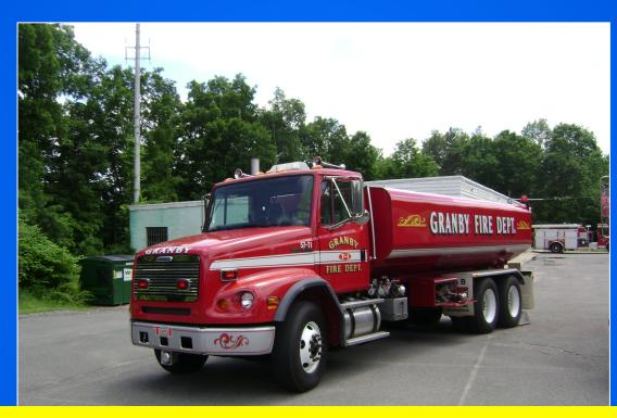
Hard to believe, but the new vacuum tanker replaces this 5,000-gallon tanker <u>AND</u>...the vacuum tanker out-performs the old tanker as well. The old tanker was slow to fill and had limited off-load flexibility and was also very close to the GVWR.
