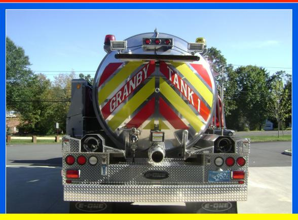
The tanker is equipped with three, 6-inch dumps — one on each side and one on the rear. When pressurized, the tanker easily can off-load its water at over 1,000 gpm through any of the dumps.
