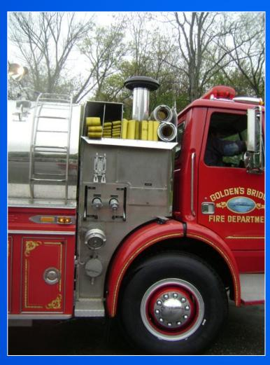
Note the 5-inch LDH loaded in the crosslay area and the 5-inch LDH discharge on the pump panel – both conveniently located for quick deployment.
