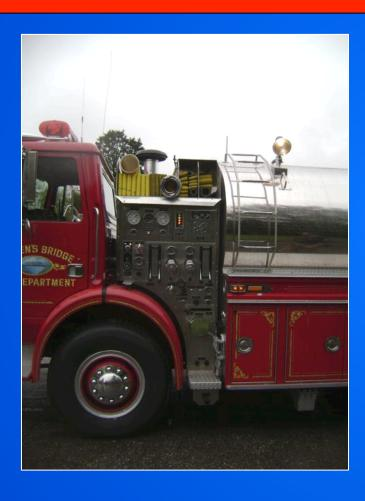
The 1,000 gpm Darley pump fits nicely into the space between the cab and the tank – although it was probably a bit of a challenge for the fellow running the plumbing! The pump allows the tanker to operate as a relay pumper, a supply pumper, or a nurse tanker if needed.
