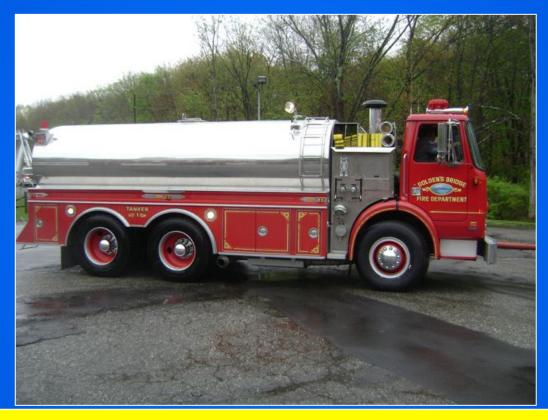
Tanker 1 is basically designed to haul water. It carries limited fire hose and equipment but it is certainly set-up to quickly load and off-load its 3,300 gallons.
