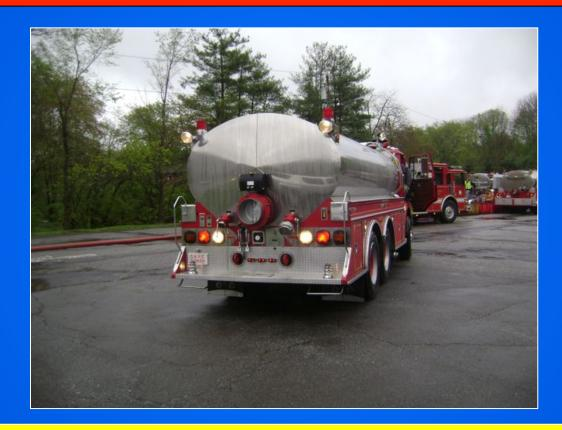
The business end of Tanker 1 has a 12-inch round dump and two, direct fill lines – one which is equipped with a 5-inch Storz fitting.
