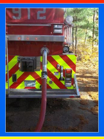
The tanker is being filled via 4-inch LDH and its 4-inch Fireman's Friend valve at the same water supply drill.
