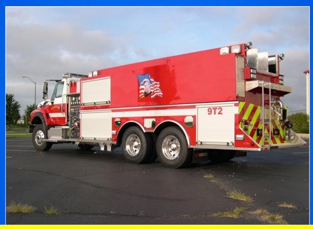
The tanker uses a "wet-side" type of design and a poly tank to carry the 2,500 gallons of water. It also has a nice amount of compartment space.
