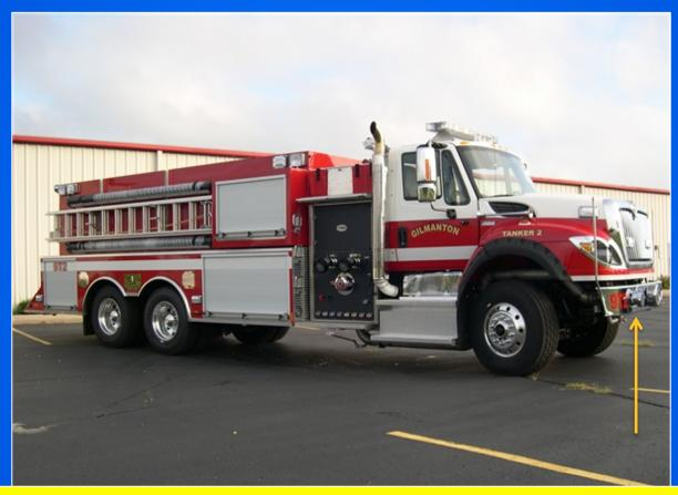
The tanker has been set up very nicely to support most any kind of water supply operation. It also has a 6-inch front suction inlet.
