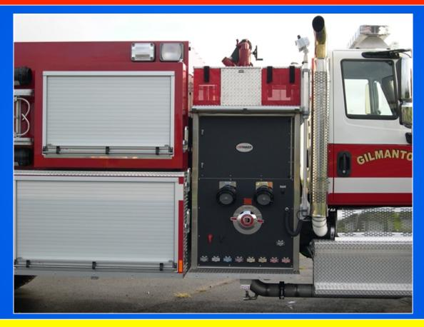
Besides having a pre-piped deck gun and a couple of cross lay pre-connects, the 1,750 gpm pump also has two, high-flow discharges.
