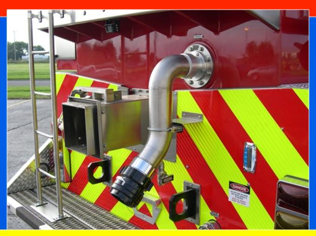
In place of a traditional control valve, the tanker uses a 4-inch "Fireman's Friend" check valve device on its 4-inch direct fill line. These valves work great and save time in the loading process.
