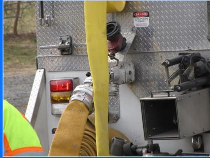
Even though the tanker has a 3-inch fill line, 5-inch LDH was used to speed-up the fill process during the drill.
