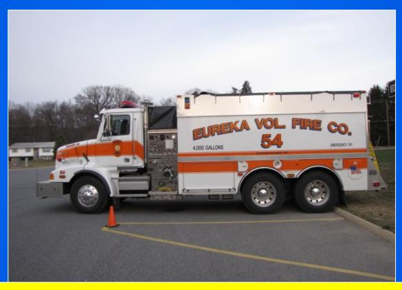
The tanker is equipped with a 1,250 gpm PTO-driven pump as well as 10-inch dumps making it quite versatile in both nurse-tanker and tanker shuttle operations.
