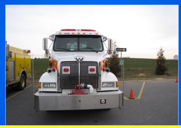
The front discharge has a short length of pre-connected 4-inch hose to speed-up nurse-tanker operations.
