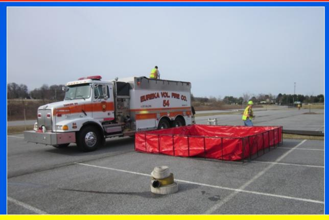
Tanker 54-1 is shown in operation above at a recent water supply drill in Harford County, Maryland. The tanker's 4,000-gallon dump tank was used at the dump site.
