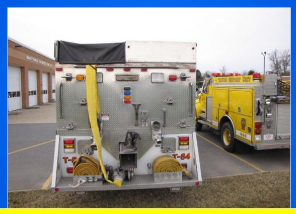
Tanker 54-1's 4,000 gallons of water can either be pumped off or dumped - or the tanker can even layout 4-inch LDH and operate as a relay pumper or a supply piece.
