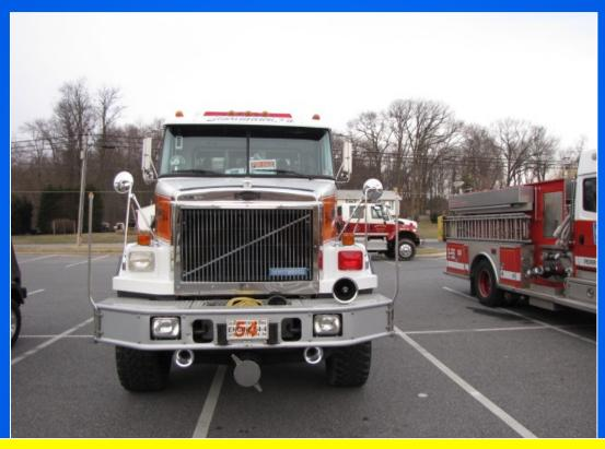
The pumper also was designed with a full-flow, 6-inch front intake that is "wyed" behind the bumper and feeds both sides of the pump's intake manifold.
