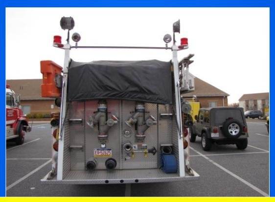
The rig's 3,600 feet of 4-inch LDH is split into two hose beds and trimmed out with the Jaffrey Z-Valve for relay pumping needs or other water supply scenarios.
