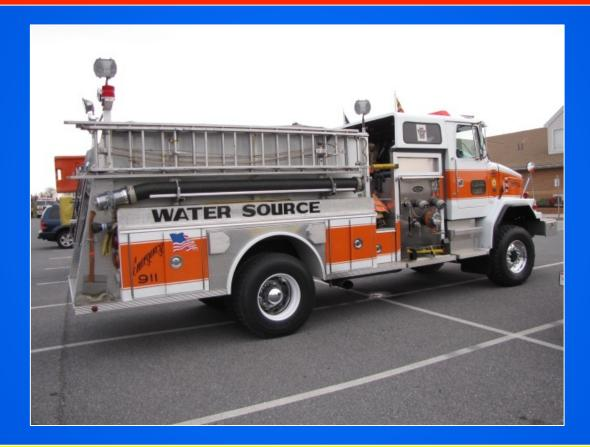
This water supply beast can pump dual, 4-inch lines from just about any position as well as be supplied by dual 4s if needed.
