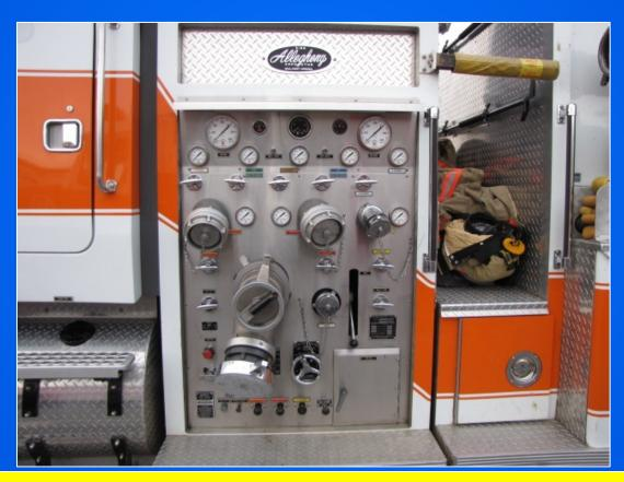
The pumper is equipped with a 1,750 gpm pump with multiple, high-flow discharges and suction inlets.
