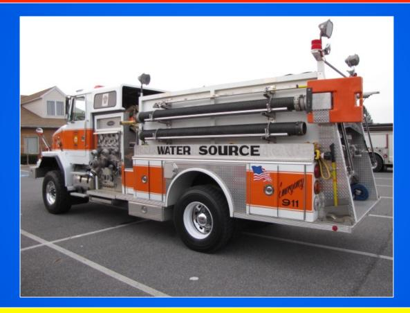
Engine 54-4 carries several lengths of hard suction hose — with some of the lengths pre-connected to suction strainers.
