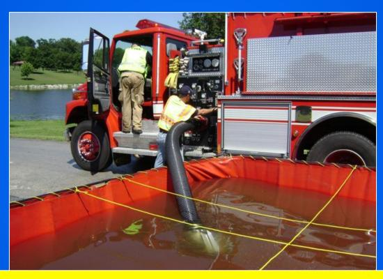
A bonus to having a 1,000 gpm pump on a tanker is that the rig can also be used as a pumper. At the 2010 drill, the dump site pumper had a mechanical issue and Tender 3 was put into operation as a pumper in order to keep the water moving.
