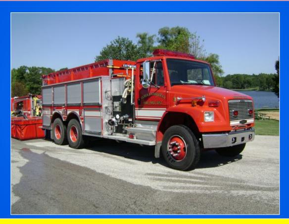
By having a 1,000 gpm pump and 3,000 gallons of water, Tender 3 provides a lot of versatility in terms of water supply operations.
