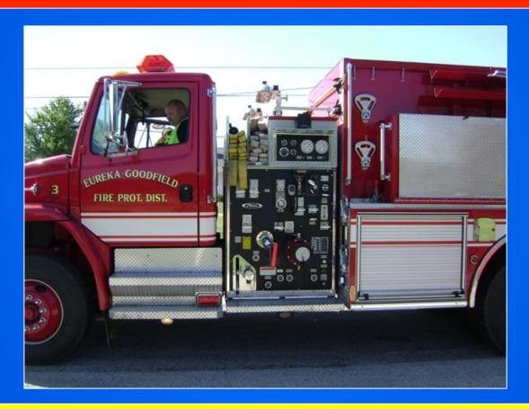
Tender 3 has a single-stage, 1,000 gpm Waterous pump and a couple of pre-connected crosslays.
