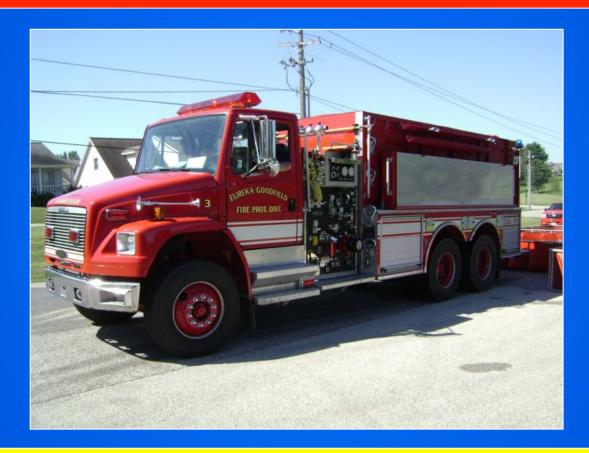
While Tender 3's primary job is to haul water, it is equipped to function as an attack piece if needed.
