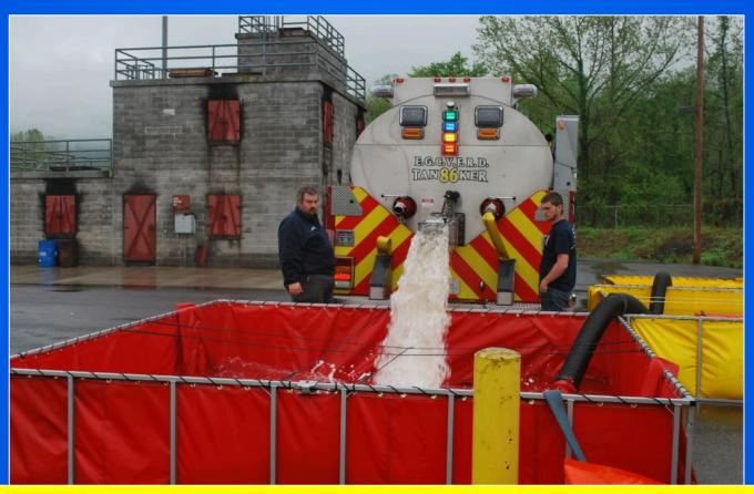
The tanker is shown here dumping its water at a training session. The 10-inch dumps allow the tanker to offload its contents very quickly.
