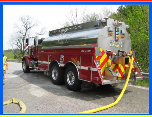
The 3,000-gallon tanker has dual, 3-inch direct tank fills and carries a variety of equipment to support water supply operations.
