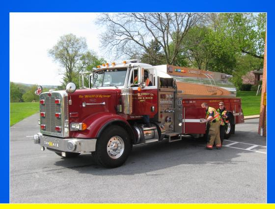
Tanker 86 is a large-capacity tanker that is designed to haul water in the mountainous terrain of Garrett County as well as along the interstate. The tanker is equipped with a 1,000 gpm pump and two, 1-3/4" crosslays.
