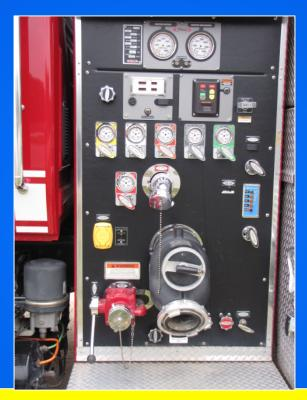
The tanker is equipped with a 1,000 gpm pump and has two crosslays. The unit is housed with an engine company and "chases" the engine in the non-hydranted areas. By having a pump, the tanker can also operate - with limited capacity - in the wildland interface as an attack piece.
