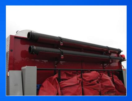
The tanker carries a 2,000-gallon dump tank as well as 20-feet of 6-inch suction hose.
