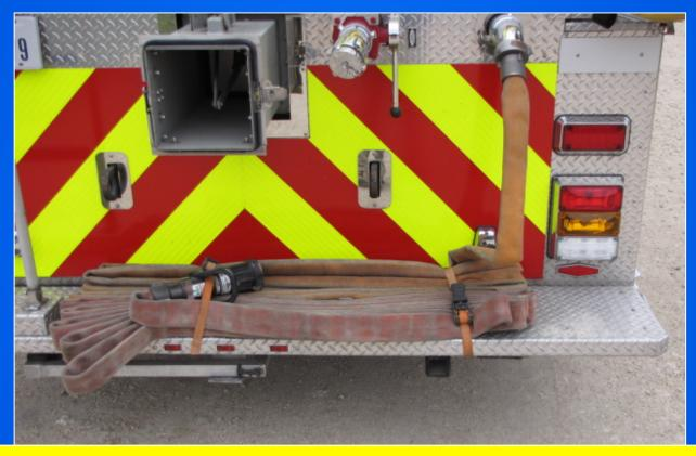
A third, pre-connected 1-3/4" attack line is stored "ready to go" on the rear step.
