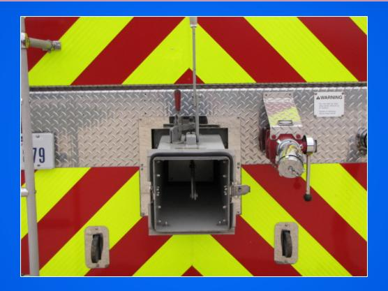
With a 10-inch rear dump, the tanker can offload its water very quickly. The rig also carries an elbow chute so that water can be dumped from the left or right side. A single, 2-1/2-inch direct fill line is used for loading operations.
