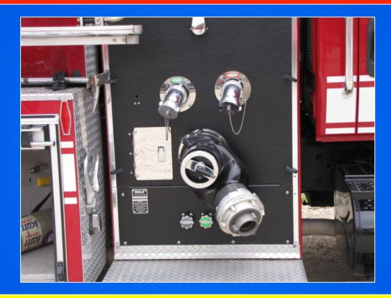
Tender 116 is equipped with intake control valves on both sides of the pump – thus providing flexibility in terms of controlling incoming water supplies.
