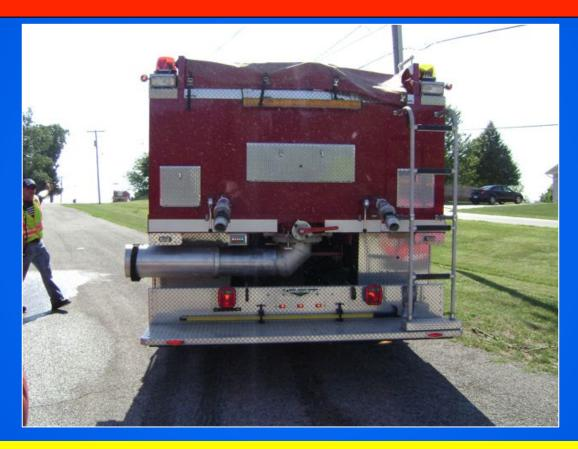
Tanker 1 is outfitted with a 10-inch round dump that swivels allowing the rig to dump from either side or the rear. The tanker also has two, 2-1/2-inch direct fill lines outfitted with camlock connections.
