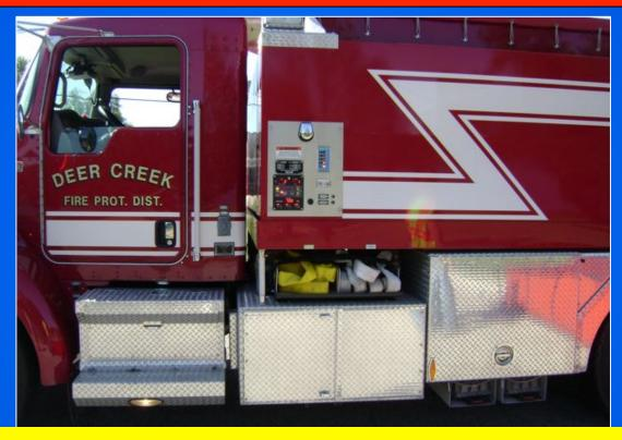
The 500 gpm PTO-driven pump is a nice feature that allows the rig to support a couple of attack lines in small fire scenarios like brush or trash fires, while also having the ability to support a 500 gpm nurse tanker operation if needed prior to dump tanks being set-up.
