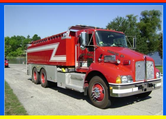
Tanker 1 is an efficient water hauling rig that is well equipped to serve as a "dump and run" tanker and as a nurse tanker as long as flows are 500 gpm or below. It could use a larger direct fill line – but the existing ones seem to work okay for most tanker shuttle operations.
