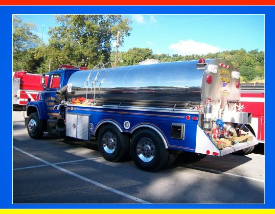
The 10-inch side dumps make the tanker more versatile in the off-loading process. Note the pre-connected direct fill lines.
