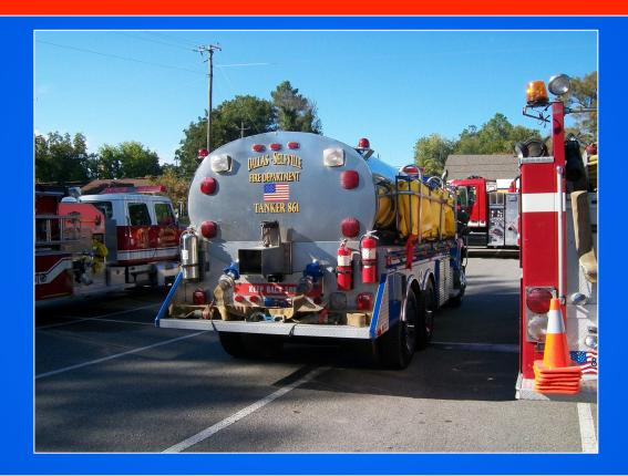
The elliptical tank design improves road handling by keeping the vehicle profile low – yet still providing adequate head pressure for fast off-loading through the side or rear dumps.
