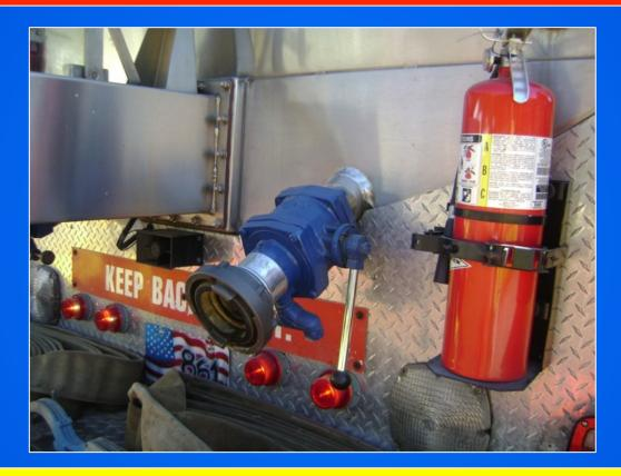
Although small in diameter, the direct fill lines are outfitted to accept 4-inch hose – which makes a huge difference in filling the tanker. Remember, a tanker loading station should work like a NASCAR pit stop!
