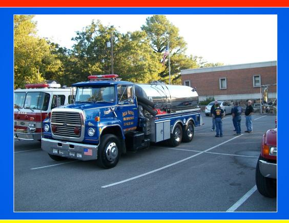
Tanker 861 is a large capacity tanker set up to operate as a water hauling unit in a tanker shuttle operation. It has a 500 gpm pump for limited, nurse-tanker and fire attack operations.
