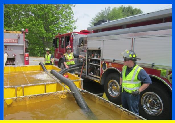
Triple suctions in use: 6-inch side, 6-inch front, 2-1/2-inch side. Water supply Chichester-style!
