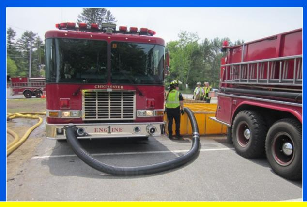
54-Engine-1 is shown here using its front intake to supplement the driver side intake so that flow can be maximized at this recent water supply drill.
