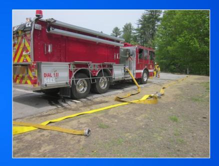
The engine/tanker carries a 3,000-gallon dump tank which really makes a difference in terms of getting water stored on the ground at the dump site. The photo above shows the engine/tanker getting ready to pump the "rural hitch" while the crew sets up the dump tank.
