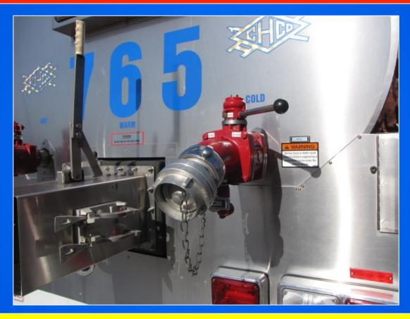
As noted many times before, the use of LDH fittings and appliances speed up the tanker filling process – without a doubt.
