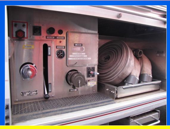
While primarily a "water hauler," Tanker 765 is equipped with a PTO-driven 250 gpm pump. The pump panel is located inside a compartment on the officer side of the rig.
