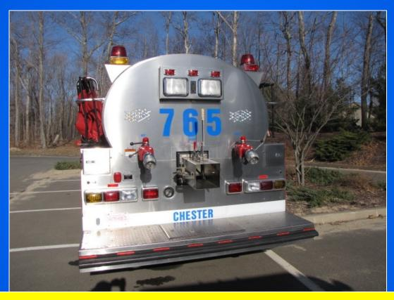
Tanker 765 has two, 3-inch direct fill lines outfitted with a 4-inch Storz connection. The Storz fitting is part of a standardization program for all tankers operated in the mutual aid association.
