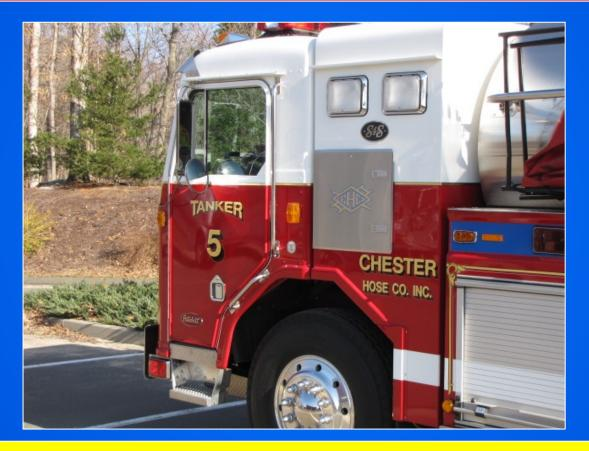
The cab-over design is one not seen often on tankers – the design helps with the short wheel base.
