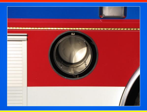
The large, side dumps are remote controlled and allow the contents to be offloaded in very short time.
