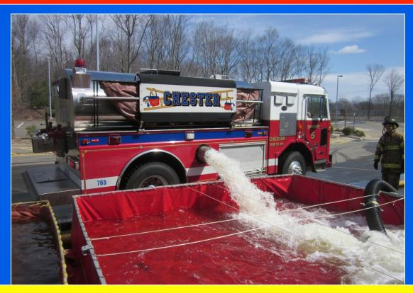
Tanker 765 is shown here dumping a load of water at a recent water supply drill in Killingsworth, CT where the folks delivered 2,400 gpm (yes, 2,400 gpm) using a tanker shuttle. Tanker 765 is clearly a great water hauling unit.
