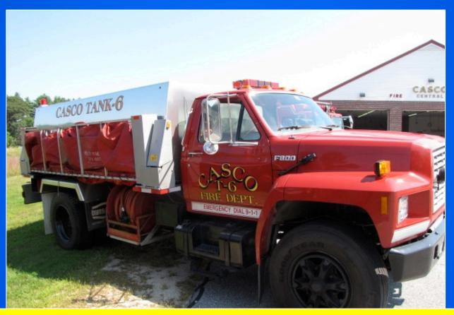
Tank 6 also has a hose reel (forestry style) and carries a 2,100-gallon dump tank.
