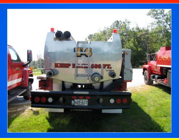
The rig has dual direct fills as well as a round dump on the rear.
