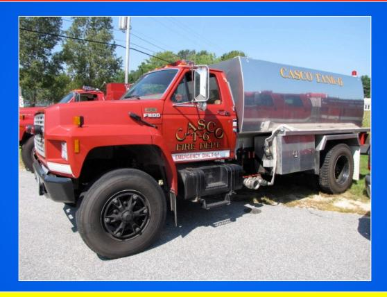
Tank 6 is a nice, short wheel-based tanker for handling the narrow "camp" roads in the lakes region around Casco.
