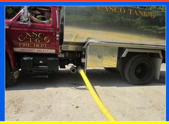
The tanker has a small, 300 gpm PTO-driven pump that allows it to serve as nurse tanker in a limited manner if needed.
