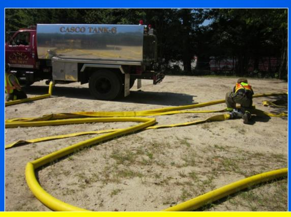
Shown here at a water supply drill in 2012, Tank 6 operates as a nurse tanker (early in the drill) and supplies 250 gpm to an attack pumper via 100-feet of 4-inch supply line.
