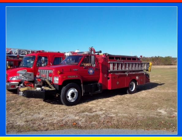
Engine 31 is equipped with a 1,000 gpm front mount and carries 1,500 gallons of water making it a pretty nice little "rural" fire fighting rig.
