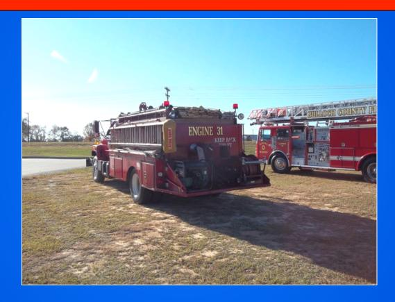
The engine/tanker has a 10-inch rear dump which allows it to offload its 1,500 gallons of water pretty fast.
