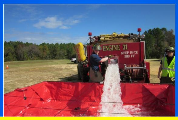
As shown here at this water supply drill in November 2011, Engine 31 is quite effective in operating in the "dump and run" mode of water hauling.
