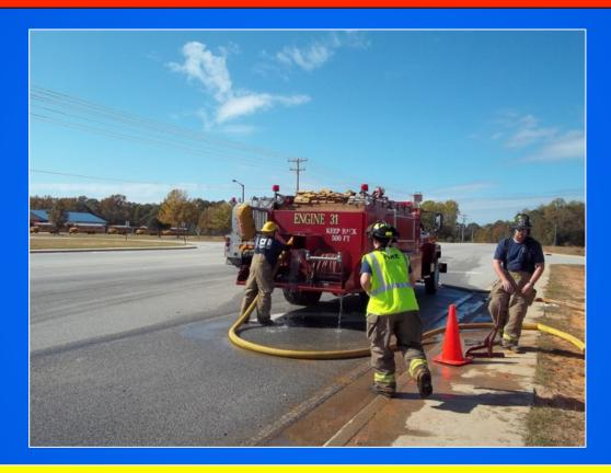
The unit has a single, 2-1/2 inch direct fill line which works okay in most instances. However, in order to fill at 1,000 gpm, a larger line would be better - or at least the use of 4-inch LDH as the fill hose.
