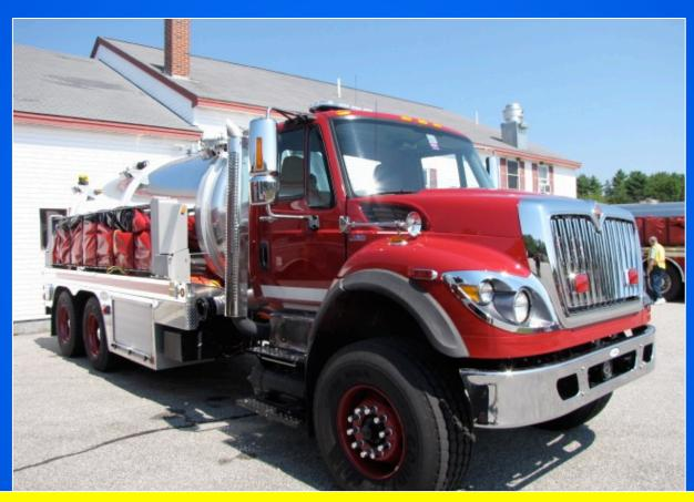
The tanker also carries a 3,500-gallon dump tank for use at either the dump site or tanker fill site depending upon how the operation is set up.
