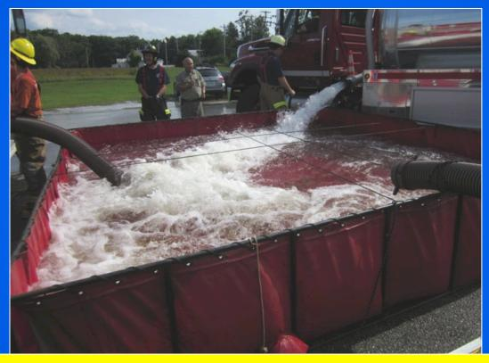
Tanker 4 is shown here offloading its 3,500 gallons at a water supply drill in nearby Casco, Maine. With the vacuum pump reversed, the tanker "blows off" its load of water at well-over 1,000 gpm.
