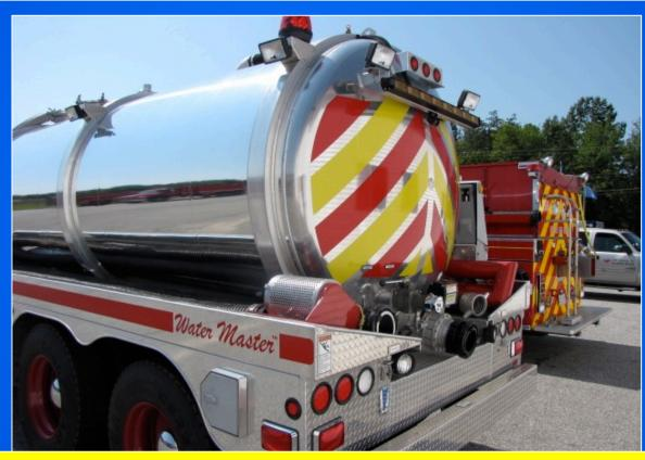
The key point about vacuum tanker operations is that no pumper is needed to load the tanker. The vacuum tanker self-loads at over 1,000 gpm!
