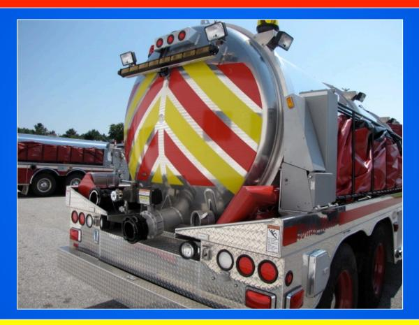
Tanker 4 carries 34-feet of 6-inch suction hose and two types of suction strainers for use in different loading scenarios.
