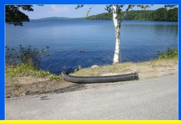
No pumper needed!!! This is what the fill site looks like for a vacuum tanker. Once the suction hose and strainer are placed – the vacuum tanker driver simply dismounts, connects the hose, and loads. Very simple!
