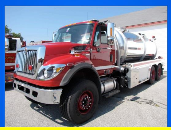
Tanker 4 is a large capacity vacuum tanker that is very efficient in water hauling operations. The rig was recently purchased by the Bridgton FD to improve water supply operations in their non-hydranted response areas.
