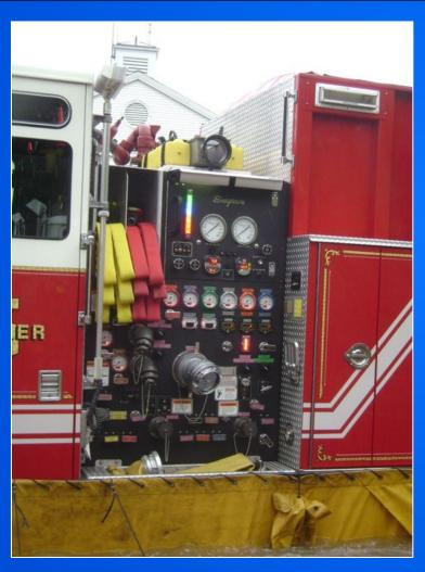
The rig's 2,000 gpm pump provides ample pumping capacity if it has to serve as an attack engine, a supply engine, or a nurse tanker.
