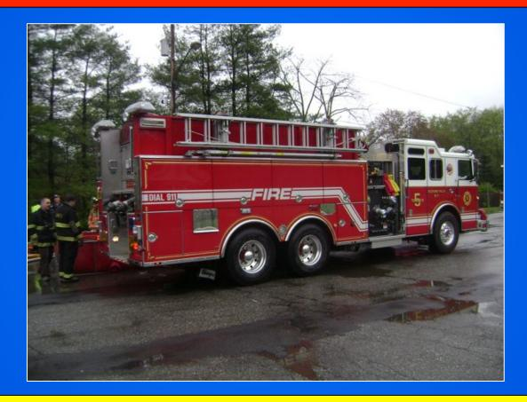
Tanker 5 also carries a 3,000 gallon dump tank in a compartment located just below the ground ladder.
