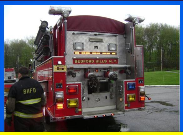
The rear end of Tanker 5 is also meant to do business as well. The unit is equipped with a 10-inch dump and has dual, 5-inch direct fills. Under that hose cover is 1,000 feet of 5-inch hose.
