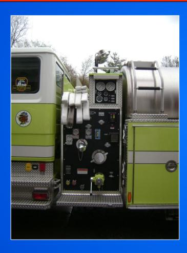
The tanker is equipped with a Hale 500 gpm pump and a couple of preconnected attack lines.
