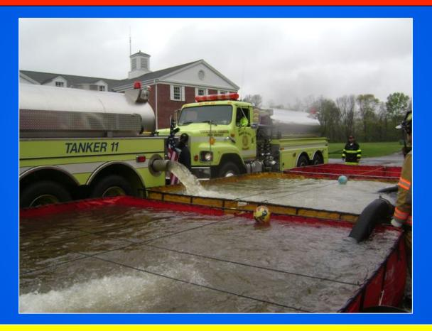
Tanker 11 is shown above at a water supply drill in nearby South Salem, NY dumping water through one of its 8-inch side dumps.
