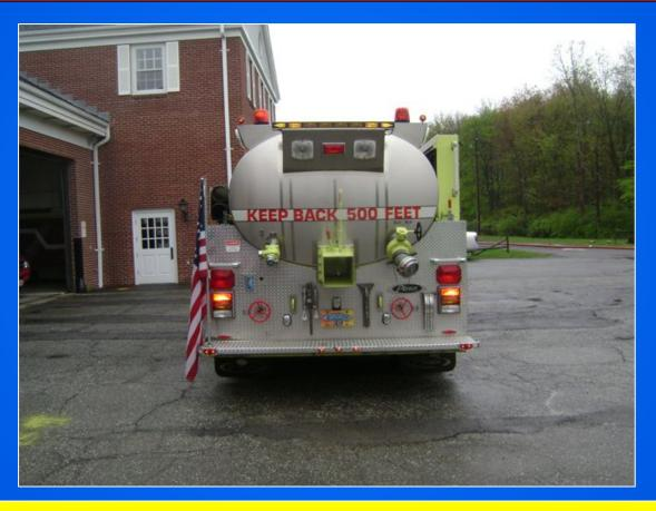
The rig has a 10-inch rear and two, direct fill lines – one of which is a 5-inch direct fill. The tanker also carries a 3,000-gallon dump tank.
