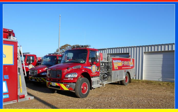
Bastrop FD operates four of these 2008 Ferrara tenders (T213, T223, T233, T243). These short-wheel-based, 2,000-gallon tenders are well-equipped to support a rural water supply operation either as a nurse tender or a shuttle tender.
