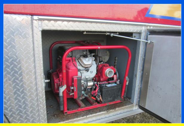
In addition to the tenders' midship pumps, each tender also carries a C.E.T 500 gpm gasoline powered portable pump. The portable pumps are outfitted to draft using 6-inch suction hose and to discharge through 5-inch LDH.
