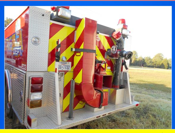
The tenders have a single, 10-inch rear dump that is controlled from the cab. An elbow chute is used to direct the water when side dumping is needed.
