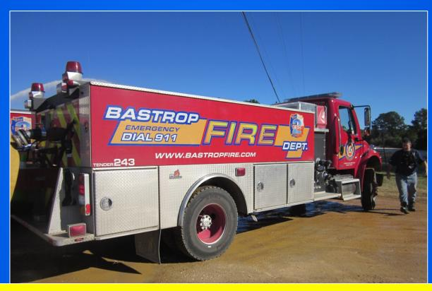
The tenders have a low profile and center of gravity which improves their handling while traveling the back country roads of Bastrop County. Each tender also is equipped with a 1,250 gpm mid-ship pump.
