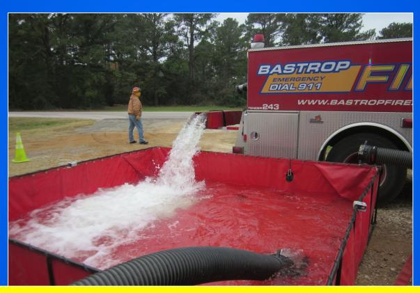
The rear "elbow" chute in action at the 2013 water supply drill. The valve is remotely operated by the driver in the cab – all of which saves time.
