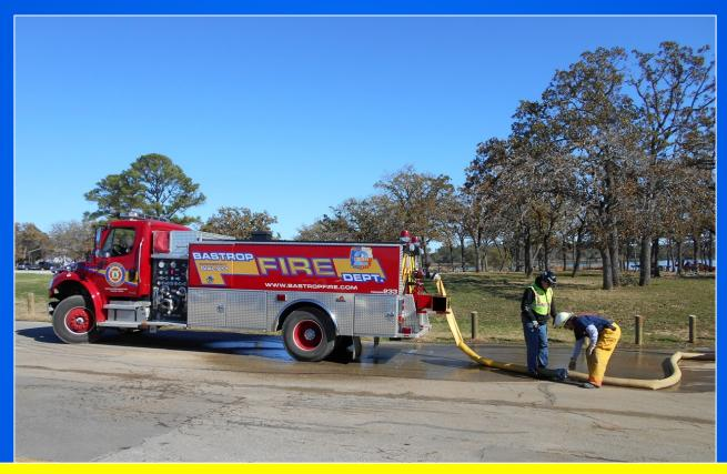
The tenders are outfitted with a rear, 4-inch direct fill line that is used to load the tenders in very little time. At this fill site operation, the Bastrop tenders were loaded at over 1,000 gpm.
