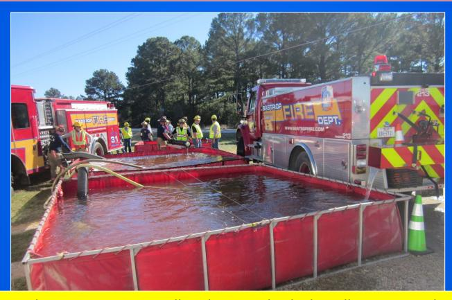
Each tender carries a 3,000-gallon dump tank which really improves the onsite storage capacity at a dump site operation. At this December 2013 drill, the first two tenders dropped their 3,000 gallon dump tanks.
