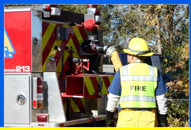
5-inch LDH is used to load the tenders. The goal is to run the fill site much like a NASCAR pit stop — and the use of LDH makes that happen.
