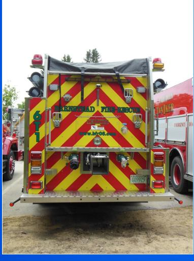
The tanker is laid out quite nicely to haul water and to support rural water supply operations. Note the three lengths of suction hose and the large, direct fill line.
