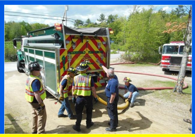
When filled using 4-inch hose, this tanker approached a 1,400 gpm fill rate!
