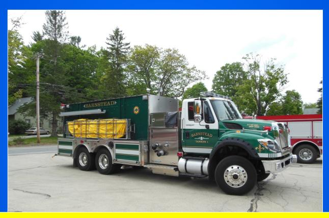
The tanker's 750 gpm pump also makes the rig quite versatile if needed to support a "rural hitch" operation or to serve as a relay pumper.
