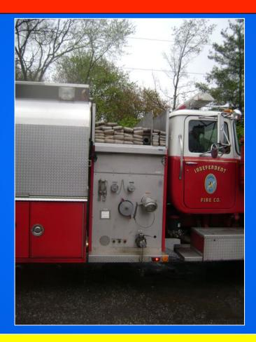
Note the LDH discharge connection – an important feature on any pump.
