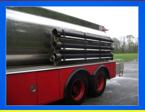
Extra suction hose is always needed in a water hauling operation and Tanker 7 carries 30-feet of 6-inch suction hose.
