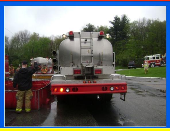
All of the dumps on this tanker are located on the rear. The rig can dump off of the rear - or the side - through any one of three, 10-inch dumps.
