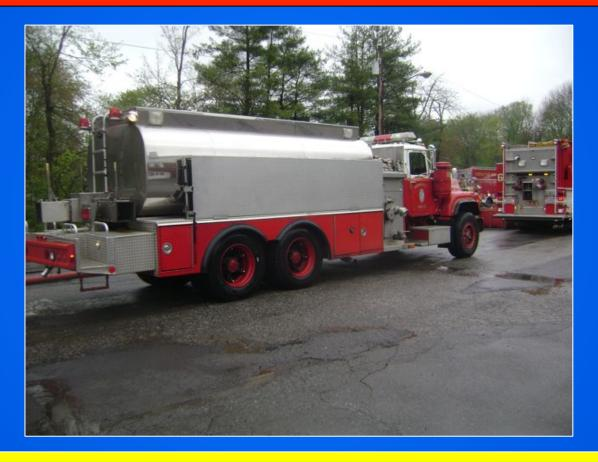
The tanker carries a 3,000 gallon portable tank and some miscellaneous water supply equipment.
