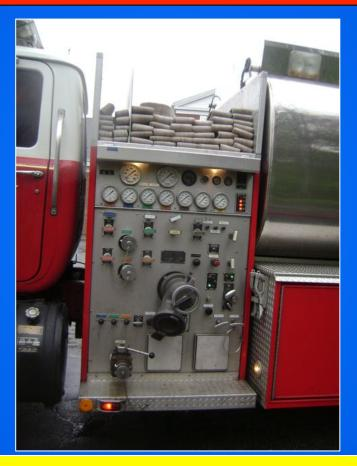
The tanker is equipped with a 1,250 gpm pump and has the ability to be supplied by 5-inch LDH.
