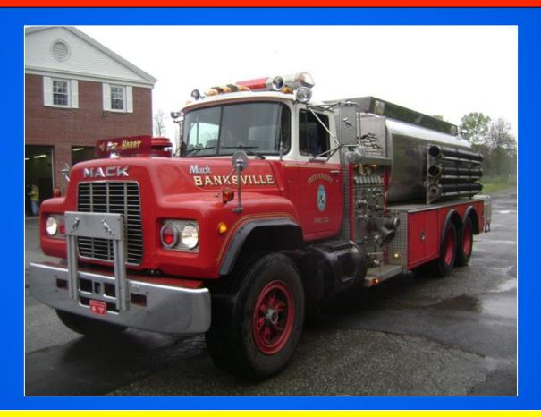
Tanker 7 is a older water hauling rig that is set up to function well in both a dump and run operation and a nurse tanker operation.
