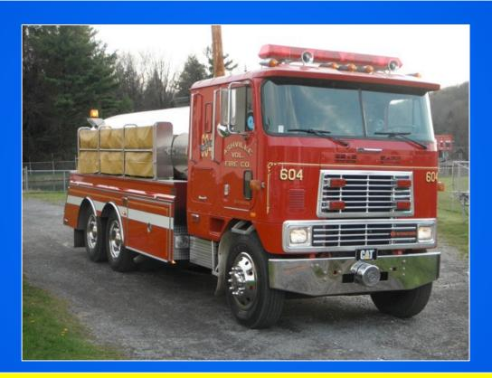
Using a chassis that once had a crane mounted on it, the department had the frame shortened, new brakes installed, a few mechanical items repaired, and a 4 Guys body built.
