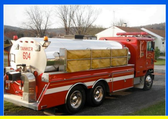
The fact that Tanker 604 is a cab-over design is simply because it was the best available option at the time. Fortunately, the department members were already accustomed to the previous cab-over tanker, so this newer model was not an issue to operate. The tanker is also short for its size, which really makes it maneuverable.
