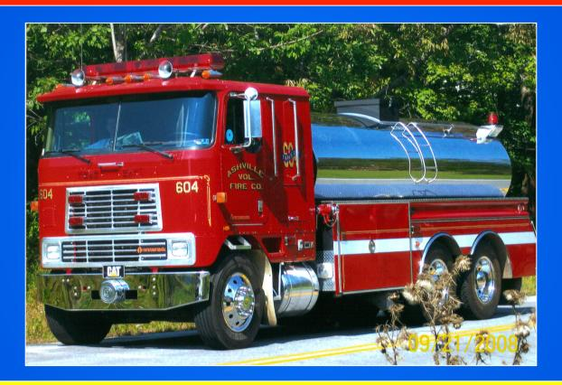
Tanker 604 is a large capacity tanker set up to operate as a water hauling unit in a tanker shuttle operation. It has a 650 gpm pump for limited, nurse-tanker and fire attack operations.
