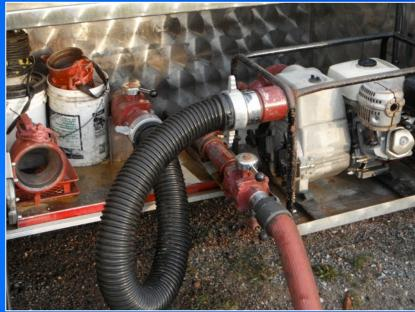
The 650 gpm pump arrangement is interesting in that the pump is stored in a compartment on a slide-out tray and uses suction hose directly connected to the tank.
