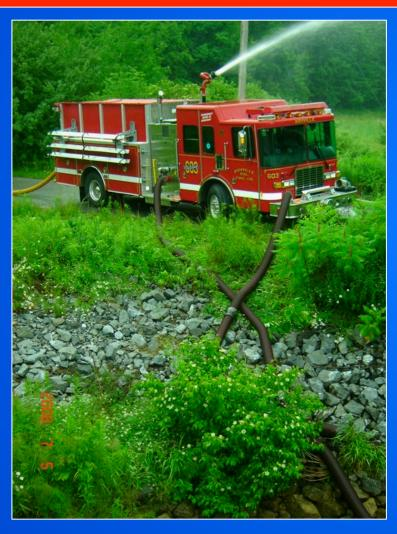
Carrying 60-feet of hard suction results in more versatility for accessing water – such as the operation shown in this photo where high flow can be supported even though the water source is farther than 20-feet from the pumper.
