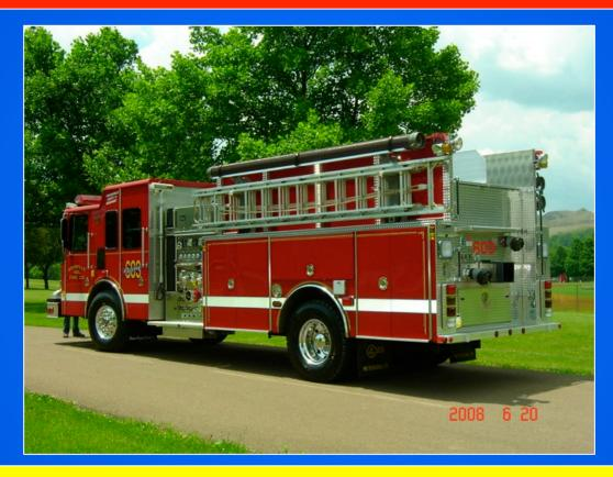
The engine is also equipped with suction intakes on all four sides of the rig in order to facilitate supporting high-flow operations.
