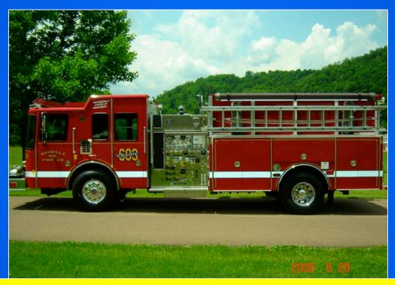
The 2,250 gpm pump is outfitted with dual primers: one traditional style primer and one custom 4-way primer plumbed to the dry side of all pump intake valves which allows for priming additional hard suctions while already flowing water.
