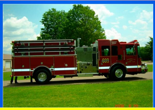
Engine 603 carries 60-feet of hard suction hose which allows it to draft using multiple inlets at the same time or draft from long distances. It also has dual, 4-inch high-flow discharges.
