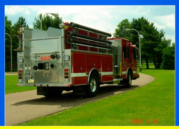
Engine 603 can also serve as a water hauling rig if need be – it is equipped with a 10-inch rear dump for shuttle operations.
