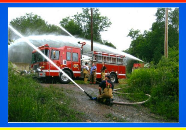
Another "big water" operation where the 2,250 gpm pump supports multiple master stream devices.
