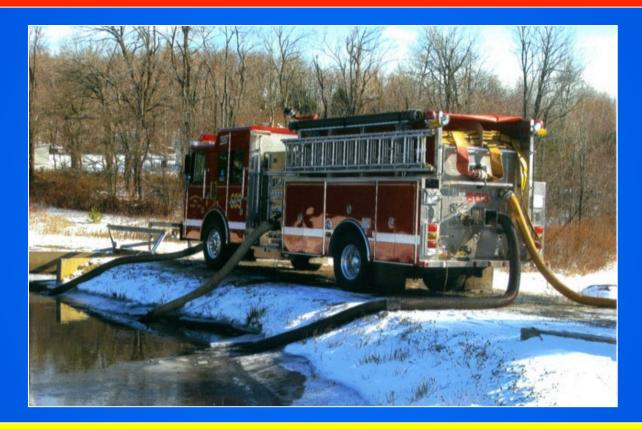
Engine 603 is shown here supporting a high-flow water supply operation by using multiple suction intakes.
