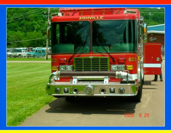
The pre-connected front suction allows for quick set-up in certain drafting applications.
