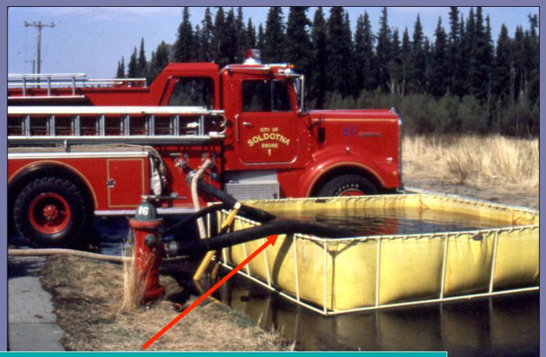
Hard suction hose is used to fill porta-tank
