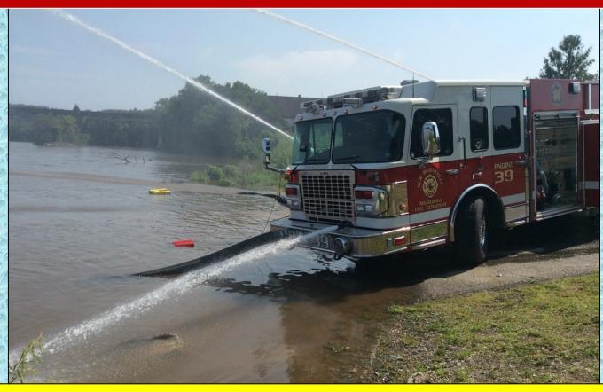
New Bridgeville Engine 39 (1250 gpm) drafted from the river using two, 6-inch suction lines and also loaded tankers at a rate in excess of 1000 gpm.
