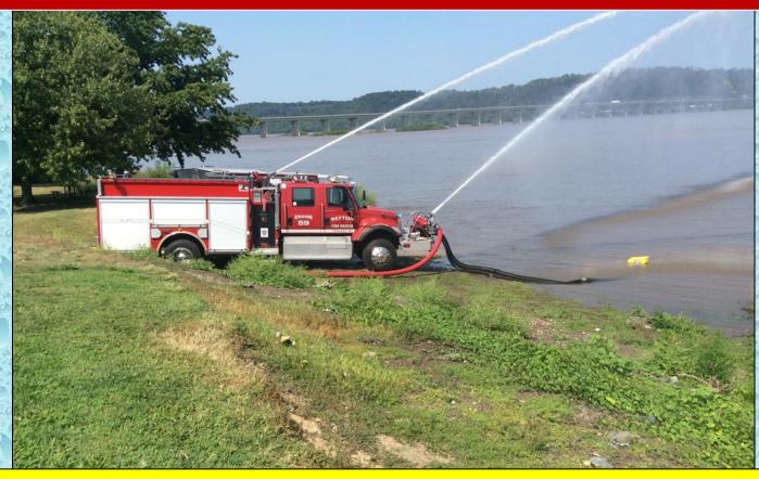
Refton Engine 59 (1250 gpm) drafts from the river using a 6-inch suction line and a 2-1/2-inch suction line. They were able to load tankers at a rate in excess of 1000 gpm.
