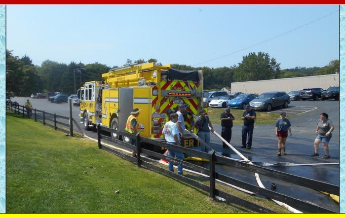
Depending on which fill site pumper was being used, tankers were either loaded using 3-inch hose, 4-inch LDH, or 5-inch LDH. Regardless of hose size, all tankers were loaded pretty darn fast!
