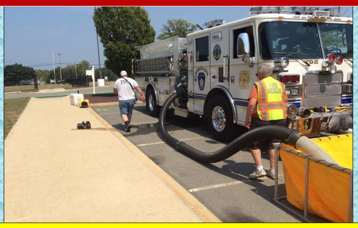
Engine 13-2 was able to deploy two, 6-inch suction lines into the primary dump tank which allowed it to pump and support the attack pumper while still supplying three jet siphons.
