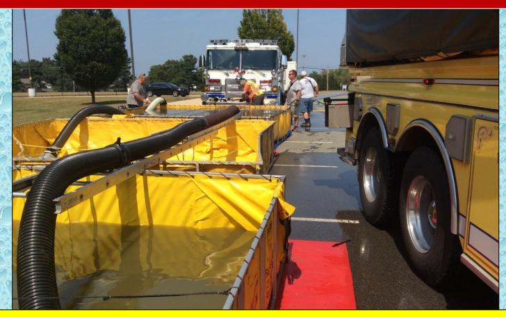
In the end, a three dump tank set-up was used to support a peak flow of 750 gpm...all supplied by one pumper.
