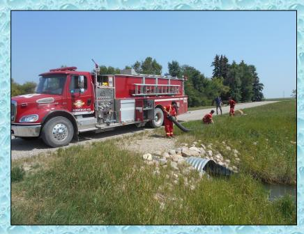
Rosebud W63 was the first unit to arrive at the fill site. Since no pumper was yet available at the fill site to help, the tender crew set-up to self-load using their mid-ship pump and 150mm (6") suction hose.
