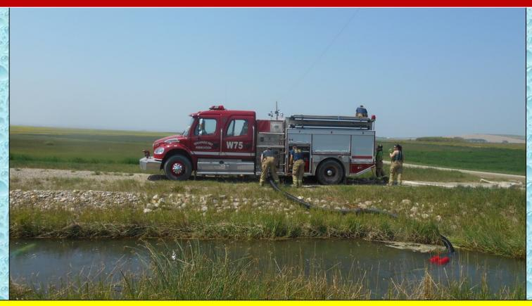
Standard W75 (4000 lpm/1000 gpm) arrived at the irrigation canal fill site after the departure of the Rosebud tender and the crew went to work setting up to draft and to build out a tender loading station. They used their 125mm (5") suction hose and a floating barrel strainer to access the canal water.
