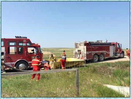
Rosebud W-63 is the next tender to arrive and takes a position to dump its water. The engine crew works to execute a "through the drain sleeve" maneuver with the suction hose and strainer.
