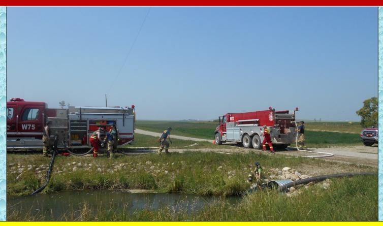
The fill site crew built out the loading area so that two, 65mm (2.5") lines equipped with camlock style connections could be used to load the tenders as they arrived.
