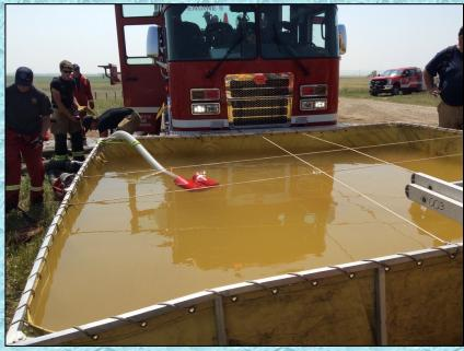
Engine 9's operator also deployed a 65mm (2.5") suction line to supplement his overall flow ability.
