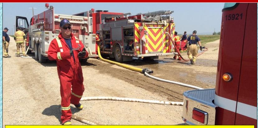
Meanwhile, a gated LDH appliance and length of 125mm (5") hose was deployed in an improvised "rural hitch" layout so that the next tender could pump off its water to Engine 9. This set-up bought valuable time while crews worked to resolve the broken suction hose problem.
