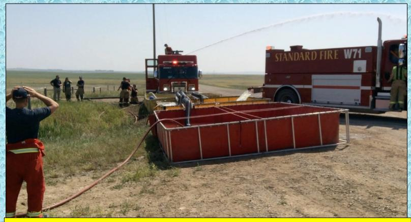
At the 72-minute mark, three dump tanks were now in operation and water flow moved to 2800 lpm (750 gpm) using Engine 9's pre-piped deck gun.
