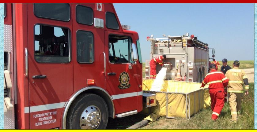
Water flow is started at 1000 lpm (250 gpm) at the 5:00-minute mark using a TFT Blitzfire and suddenly the suction hose connection fails at the pump panel. Because the suction inlet had a control valve, the operator was able to quickly switch to on-board tank water.
