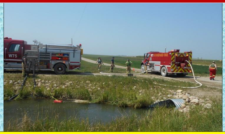
The loading station became very efficient and the crew deployed an additional suction line (65mm) to increase the supply to the pumper.
