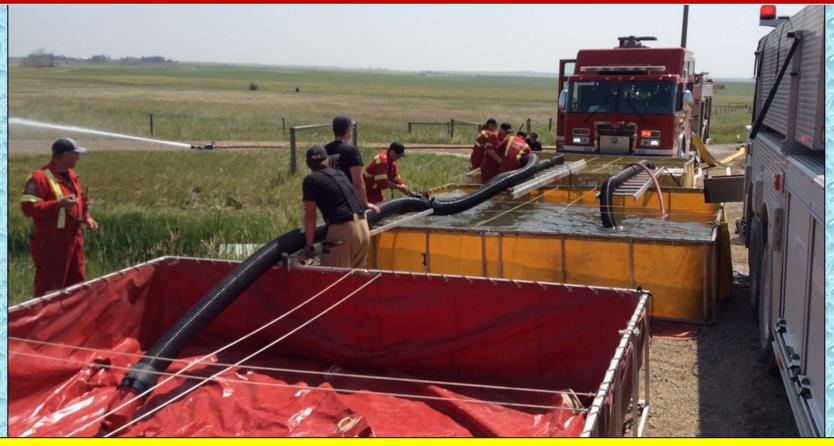
Around the 53-minute mark, crews were working to set-up a third dump tank. Part of the challenge was locating the right pieces to build out sufficient jet siphon transfer devices.
