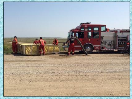
West Wheatland Engine 9 arrives on the scene followed closely by Standard W-77. Crews go immediately to work deploying W-77's dump tank in preparation for being ready to flow water at the 5-minute mark.
