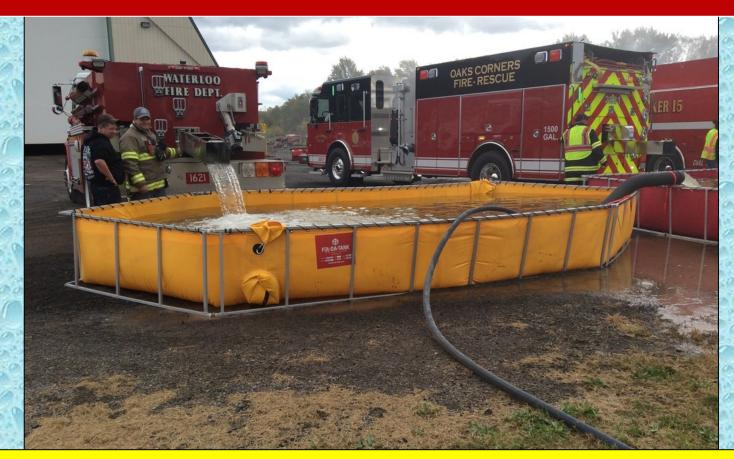
A 3000-gallon Fol Da Tank Single-Lane Type II tank was deployed as the 3<sup>rd</sup> dump tank down.
