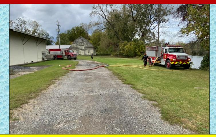
Clyde Engine 48 drafted from the river and loaded tankers using a single, LDH fill line.
