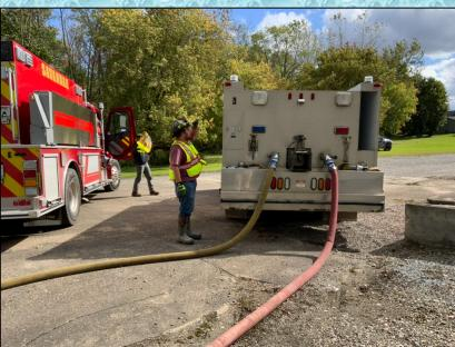
Clyde Engine 44 (1,000 gpm) drafted from the river and loaded tankers using twin, 3inch fill lines.
