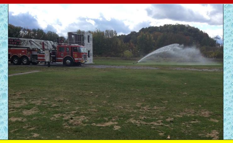
Water flow is started at 250 gpm at the 5:00-minute mark using a TFT Blitzfire. Engine 49 supplies Quint 3 with tank water while the dump site is being set up.
