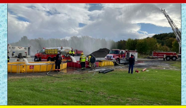
The final layout to support the 1000-gpm flow. An under-performing low level strainer in the primary dump tank was swapped out with a TFT low level strainer and Engine 49 was able to support the entire operation with much less motor work. Engine 49 also deployed a 3-inch suction line.
