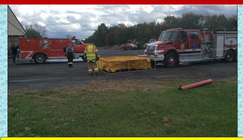
As tankers begin to arrive the crews work to set up dump tanks. A "single-lane" arrangement was chosen as the layout for this drill.
