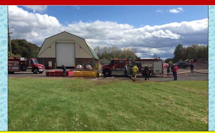
Crews work to build the dump site while still supporting the 250 gpm flow to the quint.
