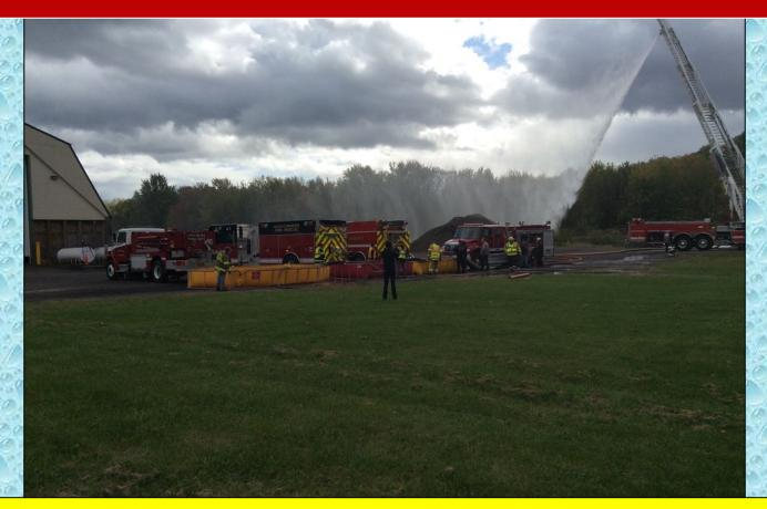
Flow was moved to 500 gpm around the 38-minute mark; to 750 gpm at the 75minute mark, and then again to 1000 gpm at the 92-minute mark.
