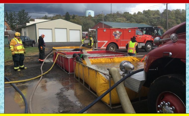
As the flow increased, water transfer operations became critical. Three jet siphon devices were used to support the 1000 gpm flow.
