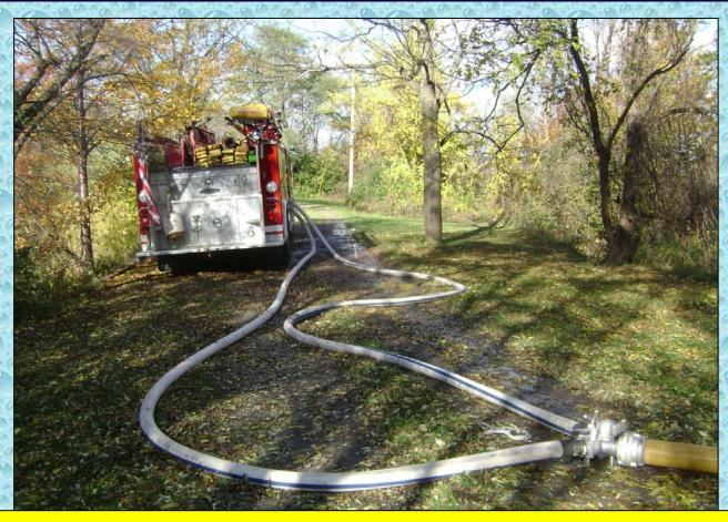
Because the pumper did not have a high-flow discharge, two, 3-inch lines were used to feed a single 5-inch line.
