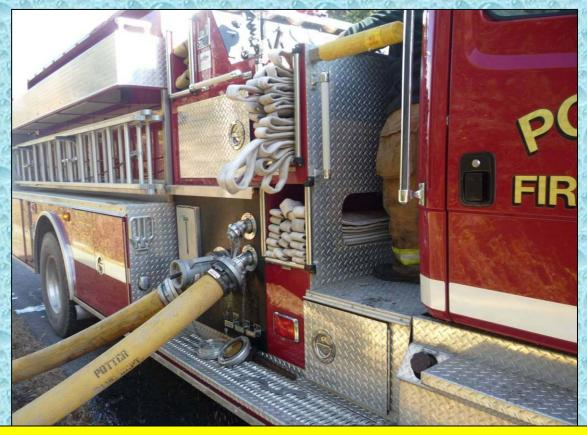
Like PT17 at the dump site, the absence of a high-flow discharge will restrict the total flow available. Perhaps a couple of 3-inch lines feeding the 5-inch line would have produced a better flow.
