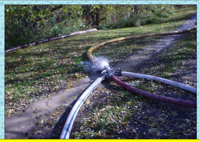
E2311 also added a third, 3-inch supply line so that the flow could be increased knowing that the goal was eventually 1,000 gpm.
