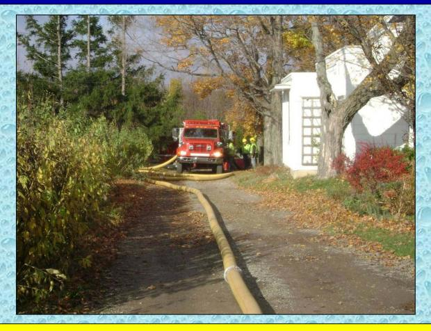
PT17 charges the 1,000 ft, 5-inch supply line feeding E16 and water supply operations begin.
