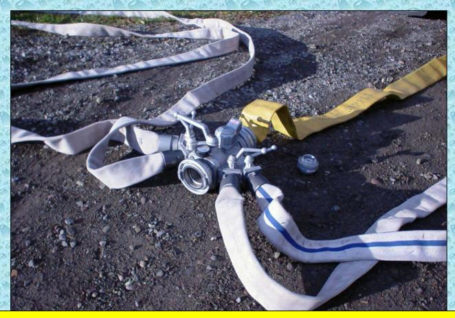
The LDH manifold makes managing the fill site much easier and takes the stress off of the pump operator.
