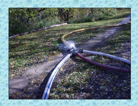
When relay pumping with pumpers that do not have high-flow discharges, it may be best to discharge two smaller lines into the larger supply line because the 2-1/2inch discharges will be limited in flow at some point.
