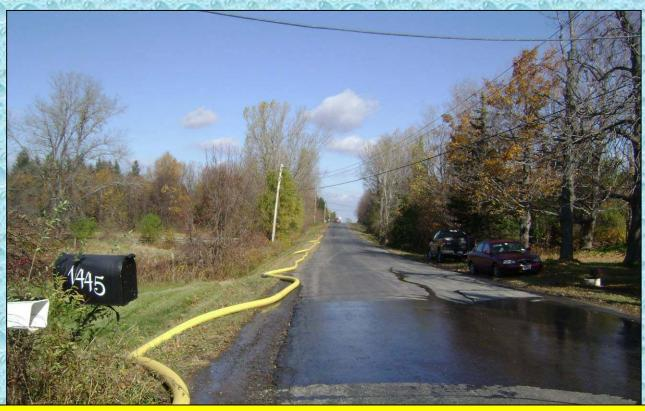
1,700 feet of 5-inch hose was laid between the fill site manifold and the dump site engine – PT17. Two tests were done – one with no relay pumper between the sites and one with a relay pumper between the sites. In each test, the goal was to maximize the flow.
