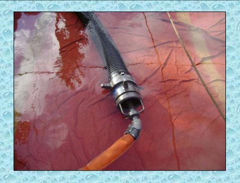
A jet siphon is used to transfer water to the primary drafting tank. One point to note is that while this type of jet siphon can really move some water, it cannot draw down the tank as low as one of the low-level siphons. Plus, this type of jet siphon often creates a vortex much sooner than a low-level type.
