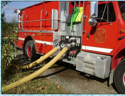
Middlesex PT17 (1,000 gpm) switched from drafting from the dump tanks to relay pumping to the attack engine, E16 (1,000 gpm). The lack of a high-flow discharge limited the amount of water that this pumper could discharge into a single, 5-inch line.
