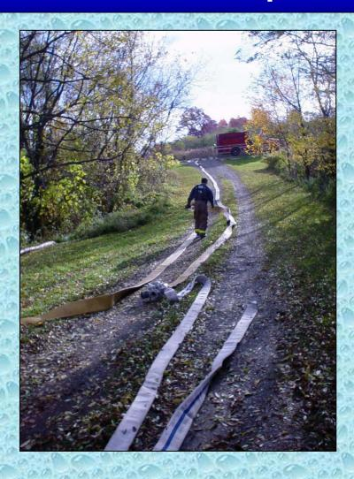
Water was sent out to the hard road via the 5-inch hose where an LDH manifold was used to control tanker fill lines.
