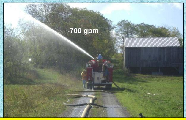
After about an hour of tanker shuttle operations, the decision was made to move to a relay pumping operation. A 5-inch supply line was laid from the tanker fill site to the dump site and the flow was increased to 700 gpm at the attack engine. (Flow was measured using a handheld pitot tube.)
