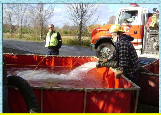
At the 10:10-minute mark, two dump tanks are set-up and water transfer operations are in place.
