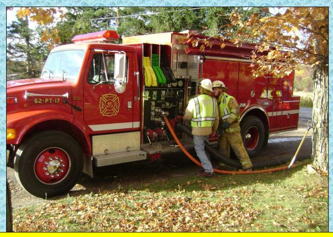
The crew of PT17 works to set up the dump site operation so that a tanker shuttle operation can begin.
