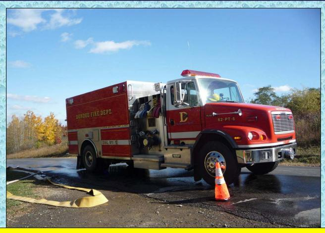
A traffic cone was used to help the driver know where to stop in order to be in the best position for the fill site crew to connect the fill lines.
