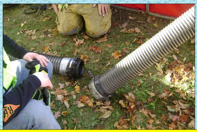
At about the 12:00-minute mark, a leak developed in PT17's suction hose. Duct tape was used as a temporary fix but since water flow was lost, the decision was made to replace the defective section.
