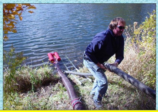
In order to improve flow at the draft site, E2311 added a third section of 6-inch suction hose and also used a 2-1/2-inch suction line.
