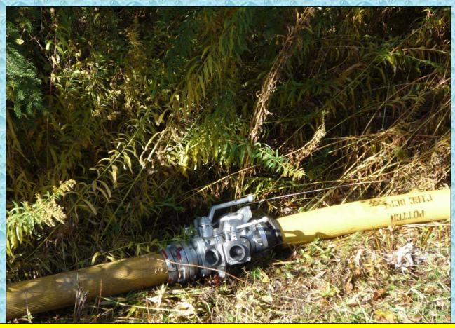
A LDH manifold was placed at about the 1,100 ft point in the line so that a relay pumper could be added later.
