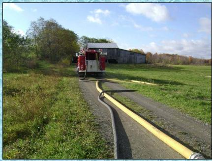
Having dumped its supply bed of 5-inch hose, Engine 16 sets up to flow water. The blue hose line in the photo is used for the initial flow of 300 gpm that was started at the 5:05 minute mark.
