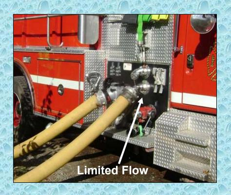
When possible, place the largest capacity pumper at the water source in a relay pumping operation – especially if that pumper has to draft.
