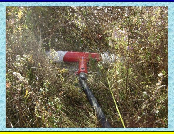
This flow diffuser - with a built-in pitot tube/gauge - was used to provide an accurate flow measurement.
