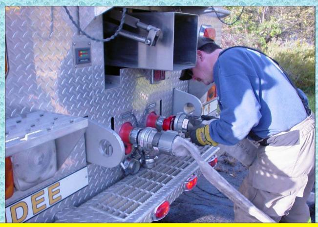
The use of Storz-style "quick-connect" fittings on the 3-inch fill lines reduced the time needed to make and break the connections.
