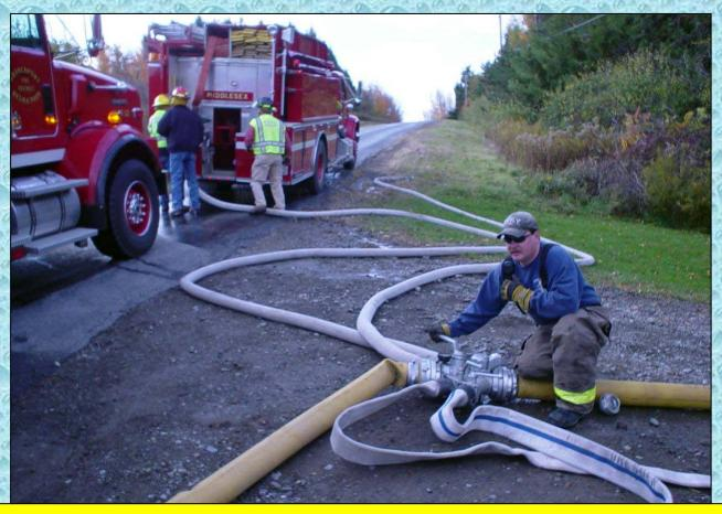
The fill site used 3-inch lines and a 5-inch line to fill tankers depending on which tanker could take which line.
