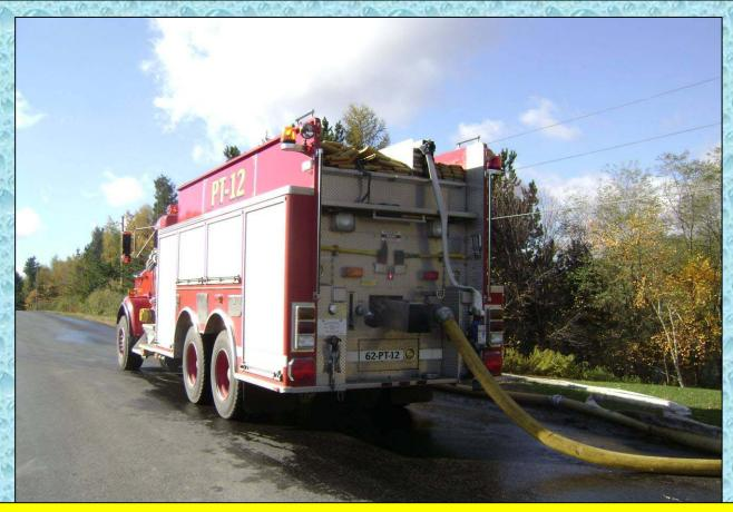
The Branchport rig was also capable of being filled through a 5-inch fill line which made filling operations go very quickly.
