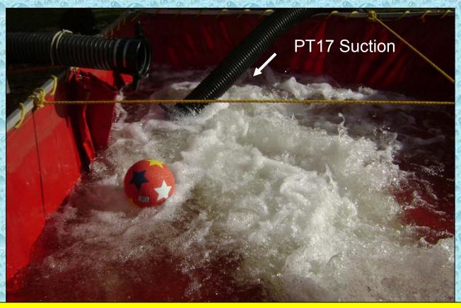
Although not always avoidable, crews should avoid tankers offloading their water directly on top of the suction strainer – it can often result in issues maintaining a prime. The playground ball it used to reduce the vortex.
