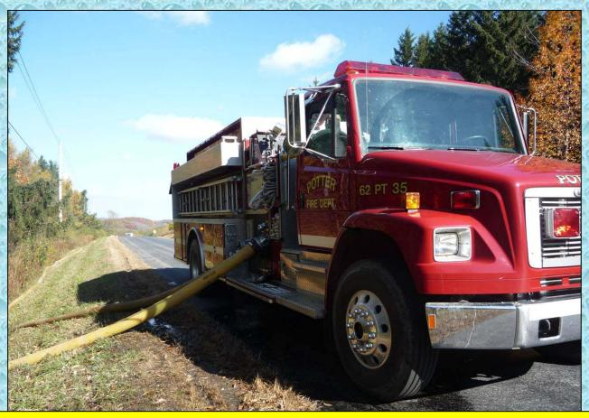
By adding this 1,250 gpm pumper, the draft pumper did not have to work as hard to move the water, thus more water could be moved.
