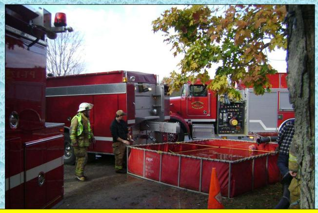
The dump site now seems to be working effectively in managing the two tank operation. However, the flow could not be increased and sustained because of the limited number of tankers in the shuttle.
