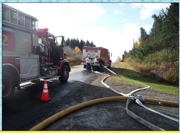
Even though two tankers were in-place and ready for filling, the fill site crews followed the best practice of only filling one at a time, thus allowing the fill site pumper to commit all of its pumping capacity to one unit.
