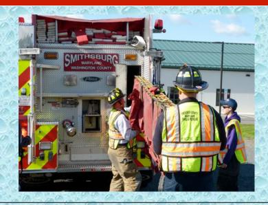
The crew of E72 set up 100' of 5" to a jumbo clappered siamese. 200' of 5" was laid from siamese to a Hosemonster which simulated an attack pumper. Washington County Tanker 7 pumped the siamese during the first few minutes of the drill while E72 set up for drafting. Tanker 7 also contributed a tank.
