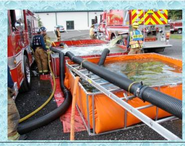
E72 was able to support up to 1100 gpm flows, three jet siphons and a circulating line. How did they do this with a 1250 gpm pumper? Three sets of suction tubes - one each from the side and front intakes with a "pony" 2.5" suction borrowed from a brush truck. This set up also nicely eliminated the flow restriction posed by the initial choice of a traditional red Kocheck low head strainer.
