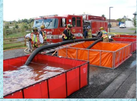
E72 set up the dump site. They used a four tank set up due to the relatively small size of the tanks. Tanks were set up far enough apart so that two tankers could dump at once. The crew did a good job of having one guy designating tanks for dumping.
