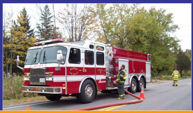
1-Engine-2 is a 2004, E-One 2,000 gpm engine/tanker with a 2,500 gallon tank. It has both a 3-inch and a 4-inch tank to pump line. The unit carries 2,000 ft of 4-inch hose. has a 6-inch rear dump/fill, and is equipped with Class A foam.
