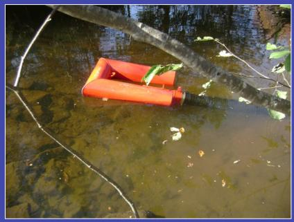
The 18 hp pump was tested first and used 4-inch suction hose and a floating strainer.
