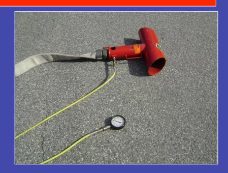
A Hose Monster flow diffuser was used to accurately measure the flow. The device has a fixed-pitot that allows for accurate pressure readings on the fixed orifice.
