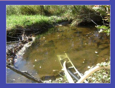
The 11 hp pump was tested second and used 3-inch suction hose and a barrel strainer.
