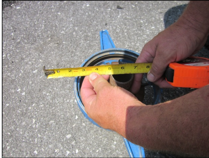
Figure 14: The Asheville Blue Thread-On siphon had a 1-1/2-inch discharge orifice – the largest of all devices tested.
