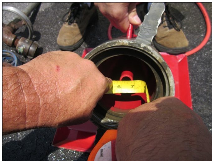
Figure 5: The 4-1/2-inch Kochek strainer had a 3/4-inch discharge orifice.
