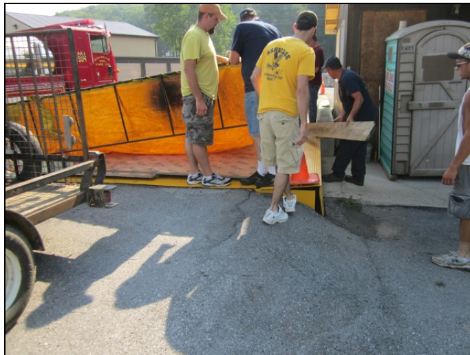
Figure 21: Tank placement was critical to obtaining accurate weight recordings.
