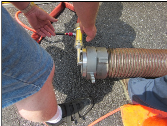
Figure 43: The Kochek 6-inch Power Jet ready for testing.
