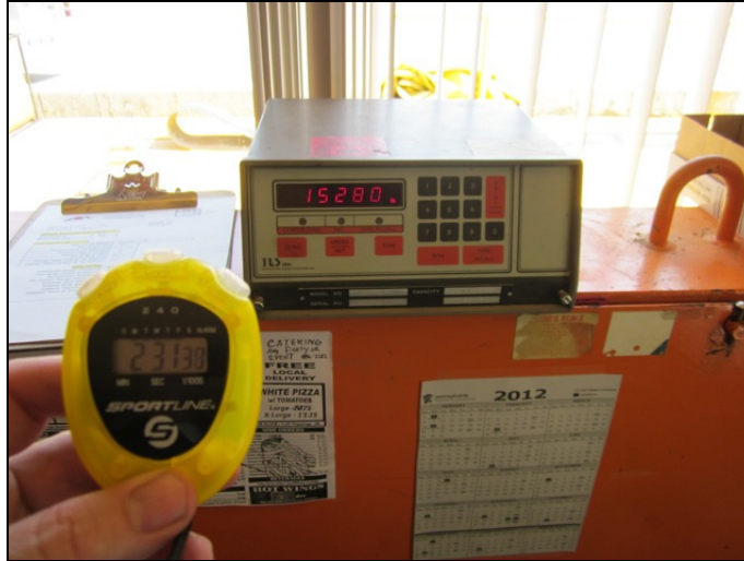
Figure 34: When the time limit was reached, a second weight recording was taken in the scale house. A flow rate was then calculated using the data collected. In this test of the Kochek 6-inch Low-Level Strainer, a peak performance flow rate of 539 gpm at 150 psi pump discharge pressure was achieved.
