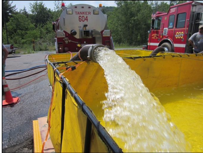
Figure 40: The Dods 6-inch Thread-In device reached its peak performance of 861 gpm at 150 psi pump discharge pressure.
