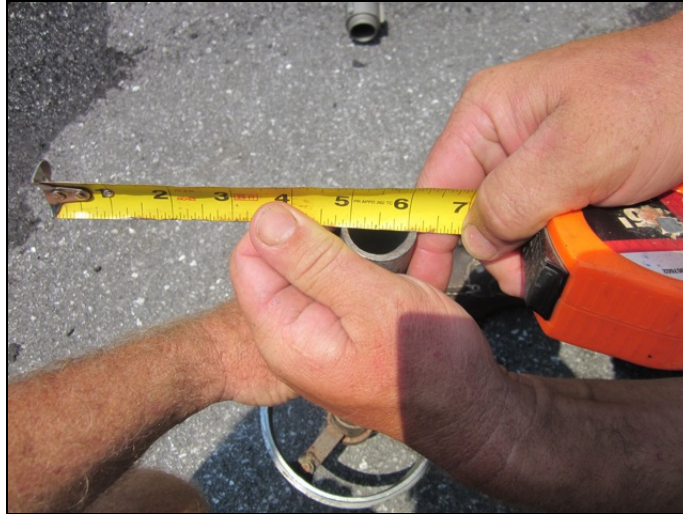
Figure 18: The Dods Thread-In had a 1-inch discharge orifice.
