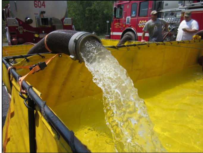
Figure 44: The Kochek 6-inch Power Jet reached its peak performance of 641 gpm at 150 psi pump discharge pressure.
