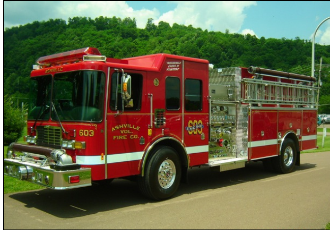
Figure 2: Ashville VFC's Engine 603 – a 2,250 gpm pumper.
