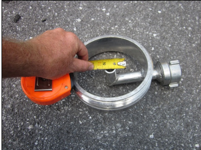
Figure 16: The Kochek Power Jet Siphon had a \frac{3}{4} -inch discharge orifice.
