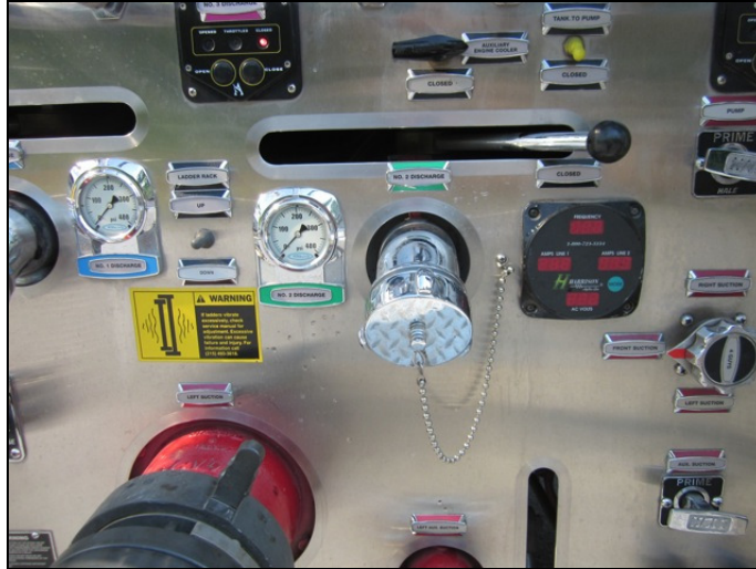
Figure 24: The #2, 2-1/2-inch discharge (green) was used to supply the jet siphon in each of the flow tests.
