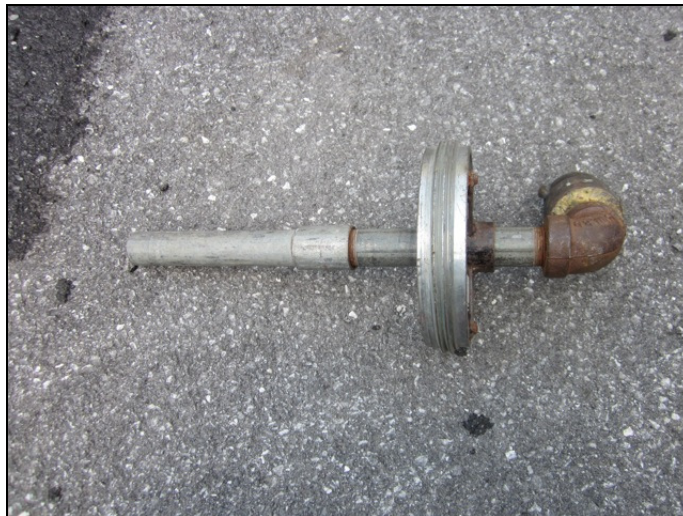
Figure 17: "Dods 6" Thread-In" (Homemade by Greg Dods, GBW Associates, LLC)
