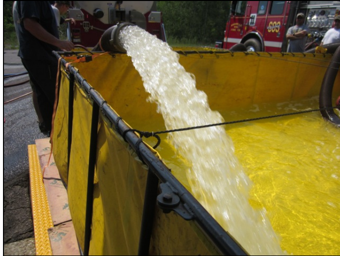
Figure 38: The Ashville Pistol device reached its peak performance of 929 gpm at 150 psi pump discharge pressure.
