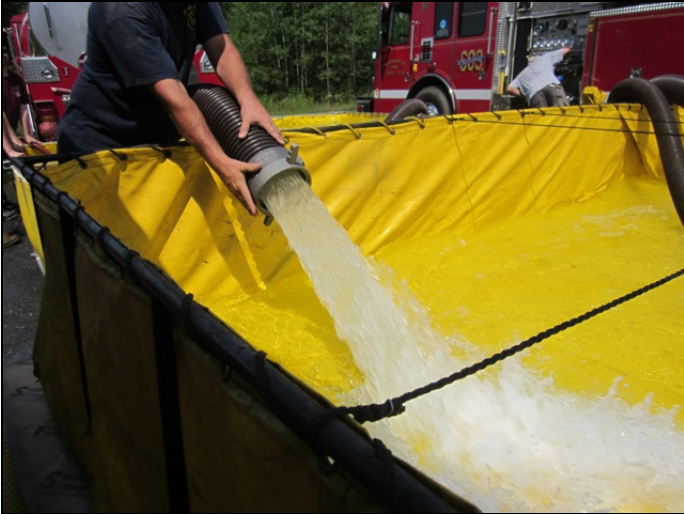
Figure 36: The Task Force Tips device reached its peak performance of 1,156 gpm at 150 psi pump discharge pressure.
