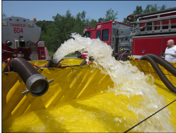
Figure 46: The Kocheck 4-1/2-inch Low-Level Strainer reached its peak performance of 556 gpm at 150 psi pump discharge pressure.
