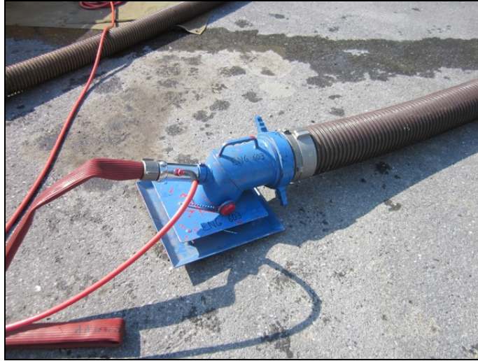
Figure 28: Each jet siphon was outfitted with the in-line test gauge before being placed in the Supply Tank. In this photo, the 6-inch Kocheck Low-Level strainer is ready for testing.
