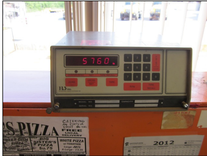
Figure 30: A “tare” weight was recorded in the scale house before water transfer operations were started.
