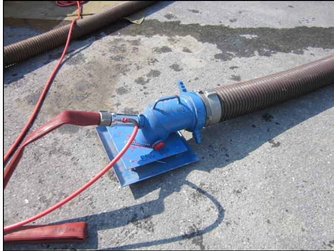
Figure 26: An in-line test gauge was placed at the supply inlet of each jet siphon to measure inlet pressure. The red air hose was connected to a remote pressure gauge for ease of obtaining and recording pressure readings.
