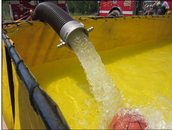
Figure 42: The Ashville 6-inch Blue Thread-On device reached its peak performance of 746 gpm at 150 psi pump discharge pressure.
