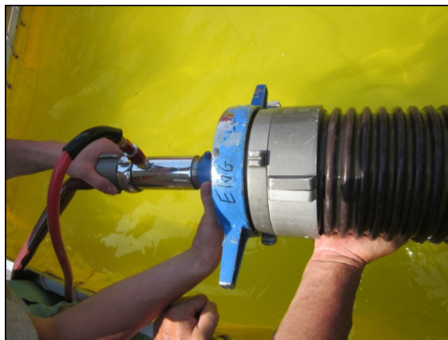
Figure 41: The Ashville 6-inch Blue Thread-On jet siphon device ready for testing.
