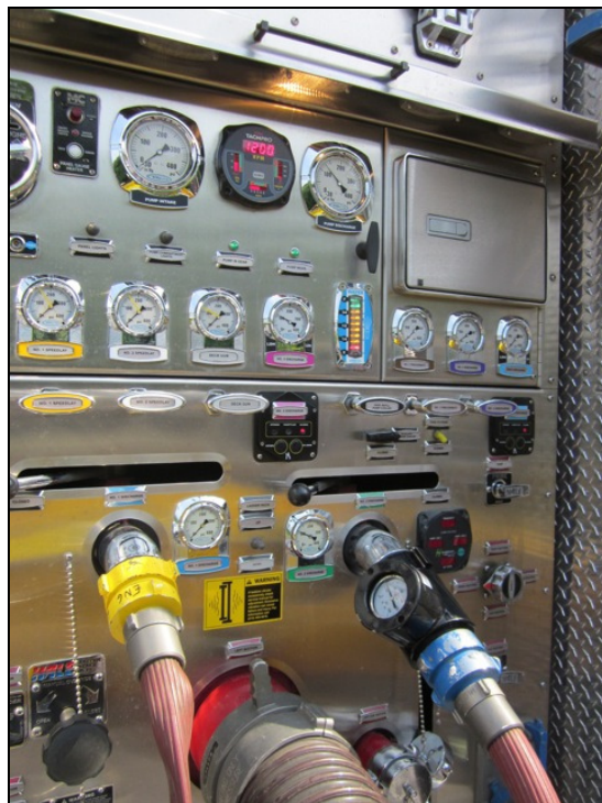
Figure 25: An in-line test gauge was used to measure discharge pressure at the pump. In all forty (40) flow tests, the in-line gauge displayed the same pressure reading as the #2 discharge gauge on the pump panel. A tachometer reading was also taken and recorded for each flow test.
