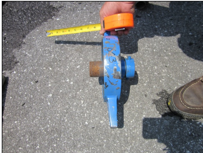
Figure 13: This jet siphon uses a very simple and unique design.
