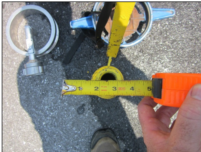
Figure 11: The Pistol had a 1-inch discharge orifice.
