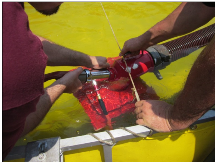
Figure 45: The Kochek 4-1/2-inch Low-Level Strainer ready for testing.
