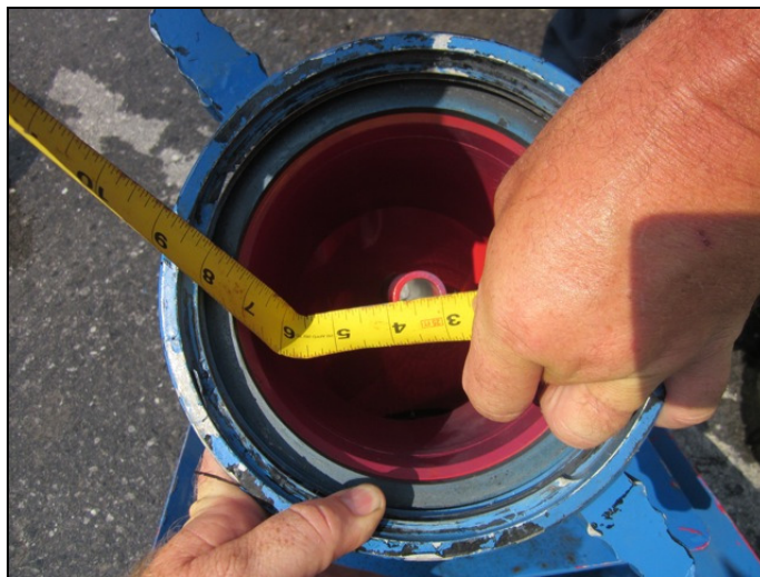
Figure 7: The 6-inch Kochek strainer also had a 3/4-inch discharge orifice.
