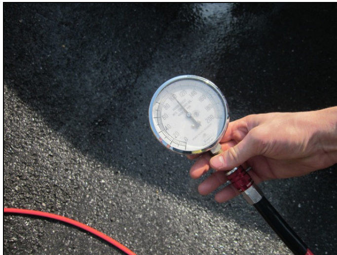
Figure 27: The remote gauge provided the pressure reading at the jet siphon's inlet.
