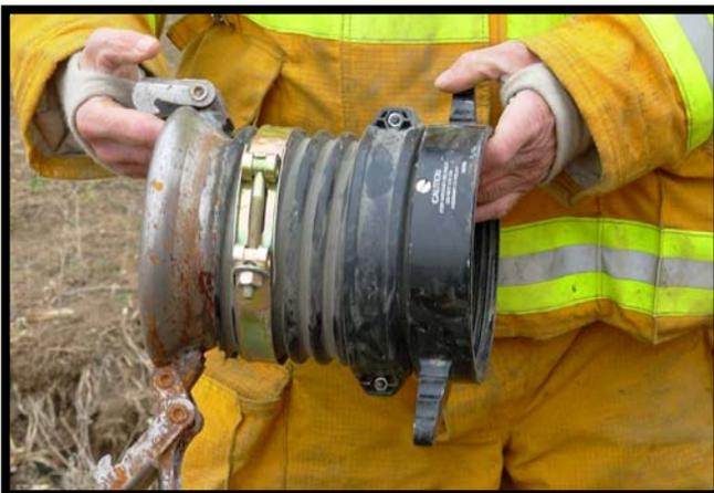
Elk Horn pumpers and mutual-aid departments carry 6" irrigation connection x suction hose adapters to allow connection to the 6" suction pipes.
