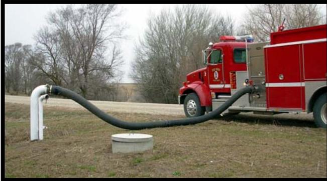
The Elk Horn VFD protects a rural area in which there are limited static water sources and one that requires the use of tankers for water supply operations. To improve water sources, department is installing 10 underground storage tanks of 6,000- to 15,000- gal capacities.
