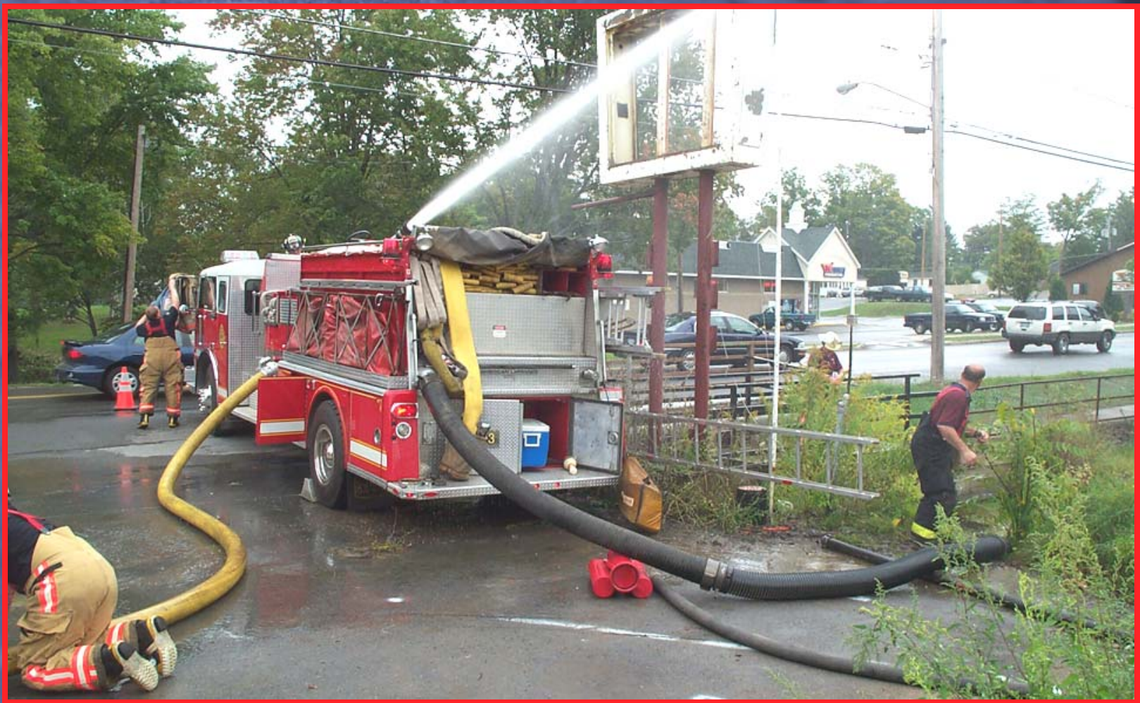
Figure 1. Drafting operations are the mainstay of the rural fire service. However, if we don't do some homework to get an idea of our pump's capabilities and what we can do to increase flow, we may in fact waste a lot of time and energy moving less water than we can with our minimum resources.
