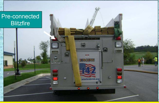
Engine 142 carries 2,300 feet of 5-inch hose plus all appliances to operate a LDH supply system. The pumper's ground ladders are located in a compartment.
