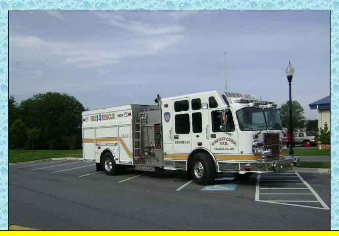
This 2007 pumper is also equipped with large flow discharges and a Harrison hydraulic generator.
