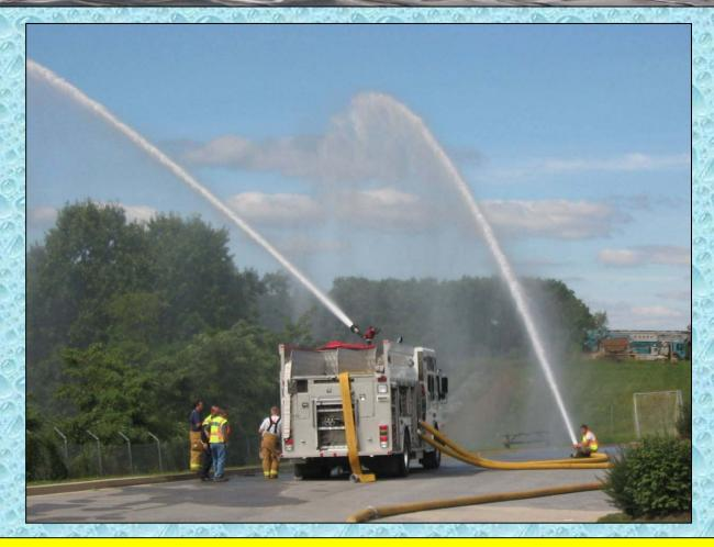
Engine 142 is shown here flowing 1,500 gpm at a 2007 water supply drill in Carroll County.
