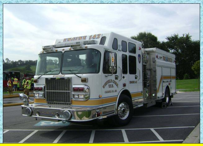
Engine 142 is set-up to operate as the "first out" pumper at Winfield. It has numerous pre-connected attack lines – including a TFT Blitzfire.
