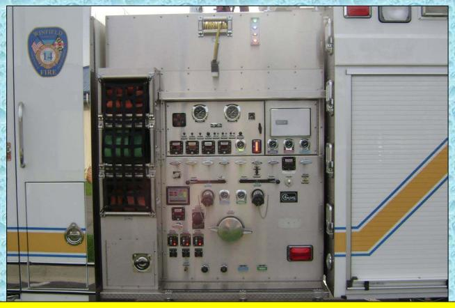
The pumper has a Hale single-stage pump and uses color-coded hose to help in hose-line selection and management. Orange is 1-3/4-inch and green is 2-inch.
