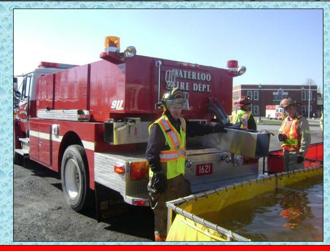
The rear dump arrangement on Tanker 1621 is quite interesting in that it allows for rear and side dumping. The tanker also has a 4" direct fill line.
