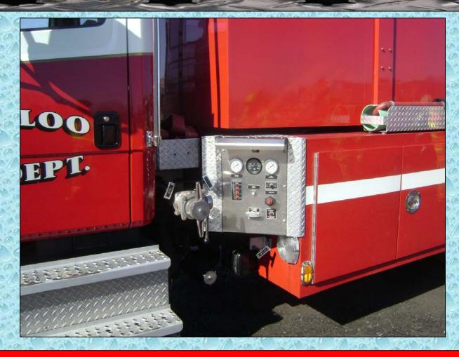
The tanker is equipped with a 350 gpm PTO-driven Hale fire pump to allow the tanker to pump off its water – of course – not as fast as dumping it.
