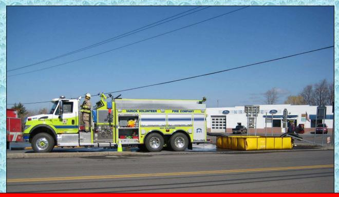
Engine 1504 is shown above working at a water supply drill in nearby Ovid, NY. The engine/tanker is drafting from a dump tank which is being kept filled by a low flow fire hydrant. By using the dump tank and the vehicle's onboard water tank, tankers up to 3,000 gallons in size could be filled at a rate faster than if they would have hooked directly to the hydrant.
