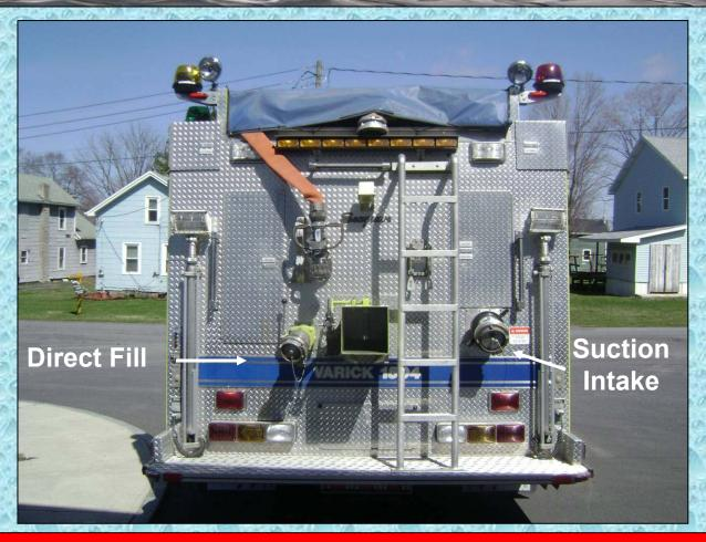
The engine tanker has a 4-inch direct fill and a 6-inch rear suction intake which also add to the rig's versatility. The rig carries 1,000 feet of 5-inch hose.
