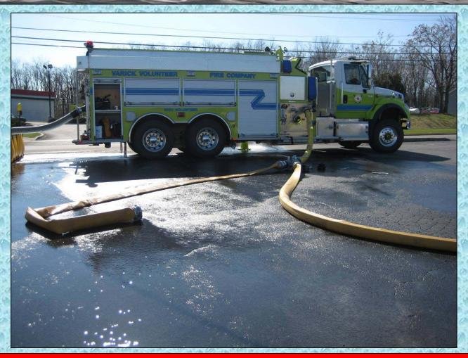
A 5"x5"x5" jumbo wye is used to operate the tanker fill lines at this tanker fill site.
