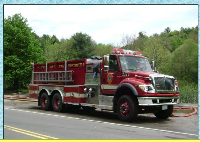
This tanker is one of several, large tankers in the region that also have a traditional, mid-ship mounted fire pump.
