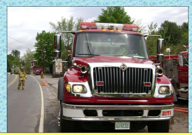
This 2006, E-One tanker is built on an International chassis and carries 2,500 gallons of water.
