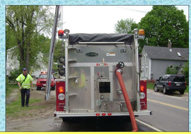
21-Tanker-1 has a 10-inch rear dump and a 4-inch direct fill line which is shown in use at this water supply drill in Ashland, NH.
