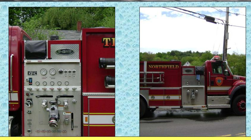
The rig has a Hale QMax, single-stage 1,500 gpm pump equipped to support the use of 4-inch LDH.
