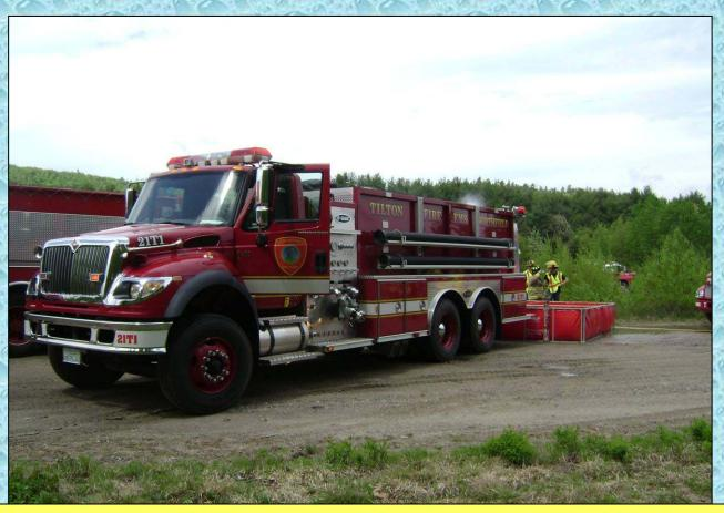
The tanker carries 15-ft sections of suction hose in addition to some basic engine company equipment.
